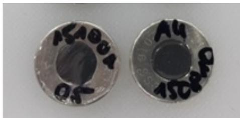
**Figure 6.4: Specially adapted coin cells; the top was covered with Mylar foil.**
