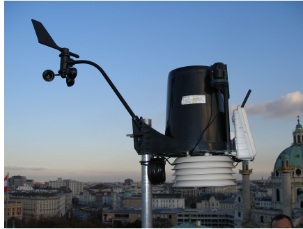
Figure 6.3: DAVIS Vantage Pro2 mounted at the TU Wien.
