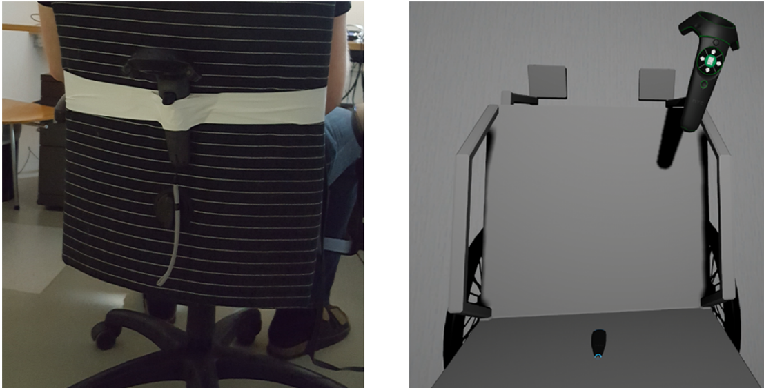
Figure 4.4: The wheelchair simulator: (left) The office chair with the mounted motion controller used for the wheelchair simulator viewed from behind and (right) the virtual model of the wheelchair in the simulation viewed from above.
