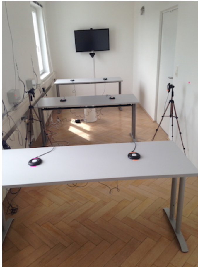
Figure 5-3. Arrangement of illuminance meters in the test room (Photo credit: Ghazal Etminan)
