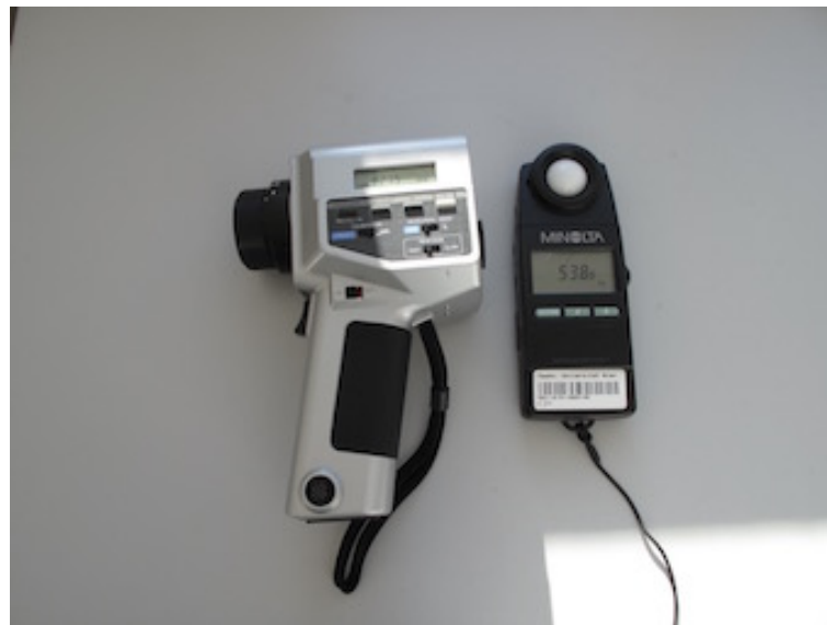
Figure 5-2. Minolta luminance meter ( LS-100 ) (on the left) and illuminance meter ( T10-A series ) (on the right)
