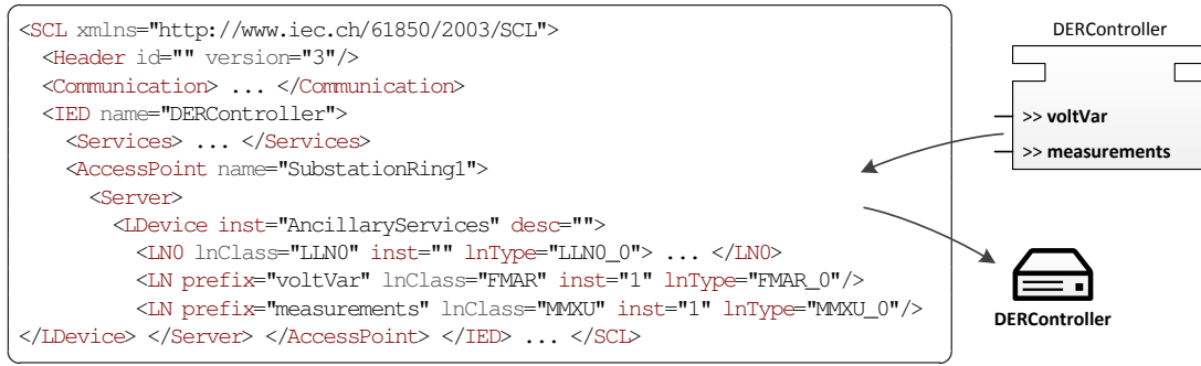
Figure 6.10: Generated SCL file for configuration of the IEC 61850 server in DERController .
