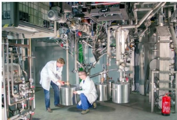
**Figure 12: Pictures of the novel DFB reactor system without thermal insulation (Left: upper reactor parts and hopper system, Right: lower reactor parts)**
