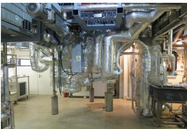
**Figure 13: Pictures of the novel dual fluidized bed reactor system with thermal insulation (Left: upper reactor parts and hopper system, Right: lower reactor parts)**
