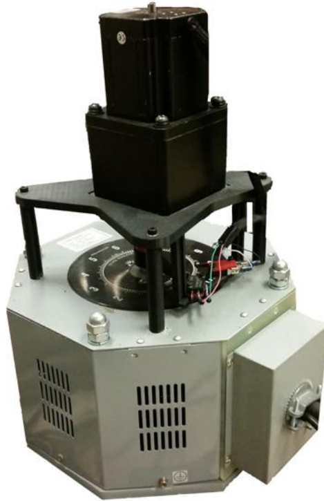
Figure 3-7: Remote controlled transformer to adjust the heating element voltage.
