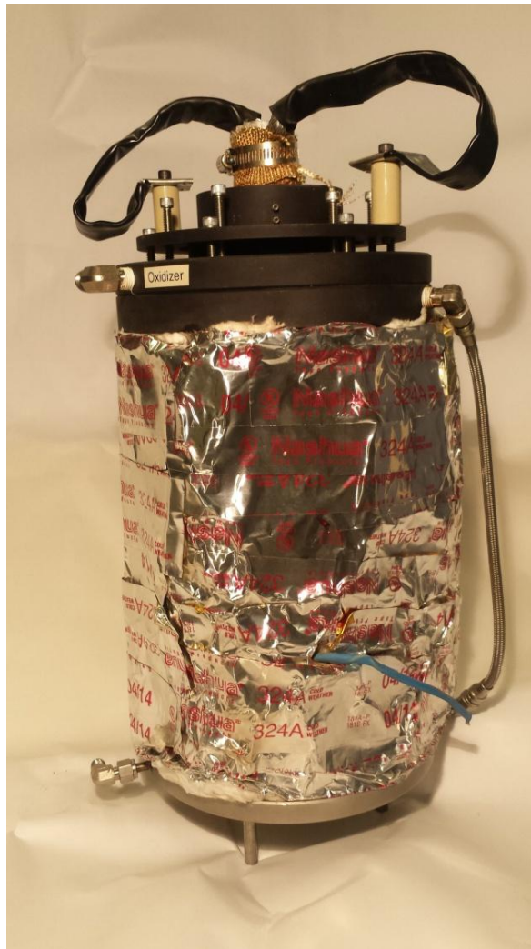
Figure 3-14: The "autoignition top" for elevated pressures.
