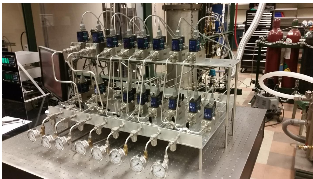
Figure 3-19: HPCEF mass flow controller setup.
