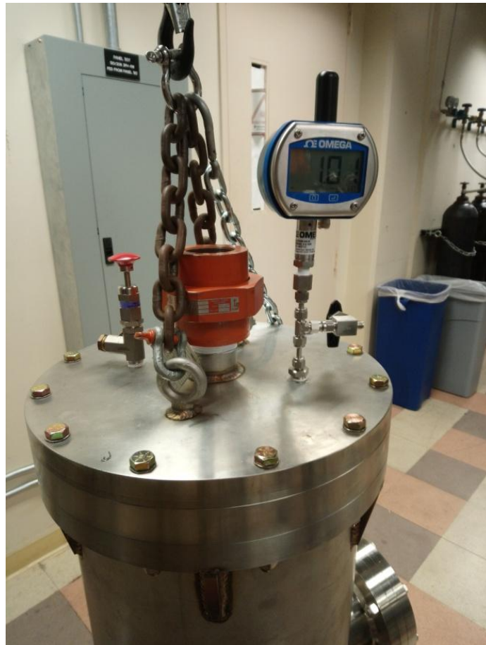
Figure 3-12: Upper part of the pressure chamber with the safety devices.
