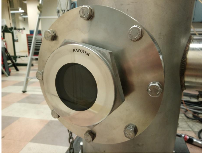
Figure 3-11: View port with the glass insert and the adapter plate.
