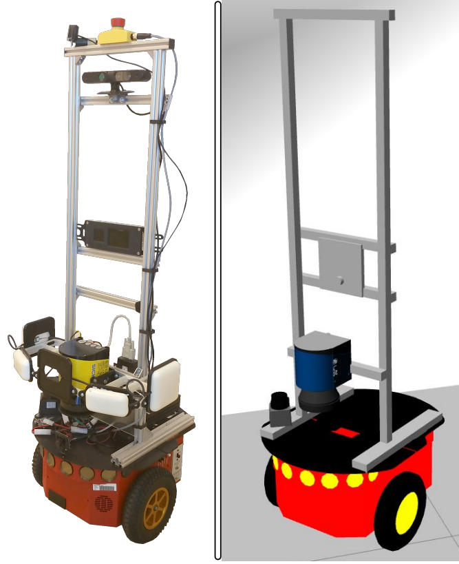
Figure 6.1: Robotic Platform Pioneer-3DX (left) and its simulated model (right).
