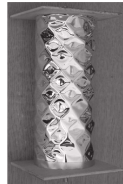
Fig. 4.5.03: Surface texturing through cylindrical buckling
