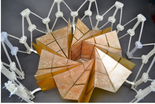
Fig. 4.01: Solar array NASA testing folding prototype
