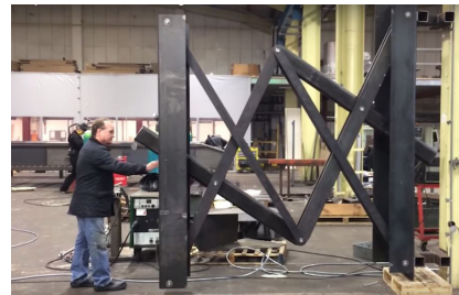
Fig. 4.1.16: Ten Fold Technology scissors mechanism - testing prototype
