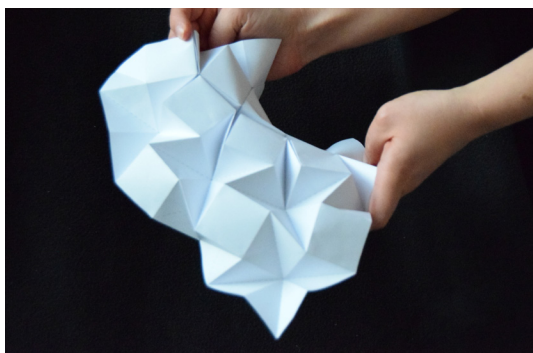
Fig.4.3.12: Deformation into curved surface
