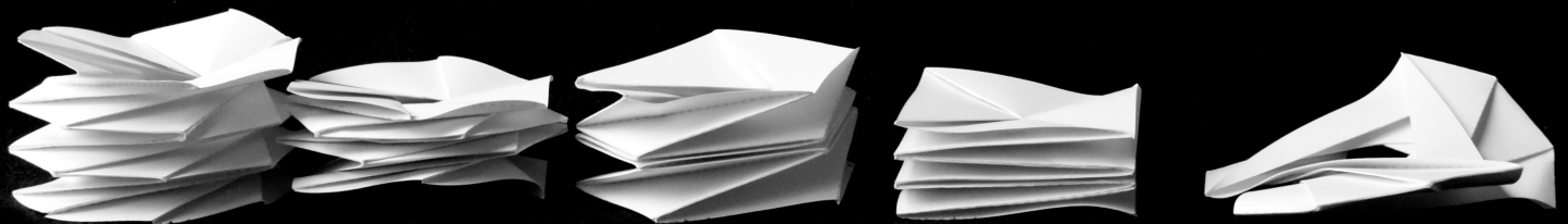
Fig. 4.5.01: b) Kresling pattern with different polygonal shapes - flat folded tubes
