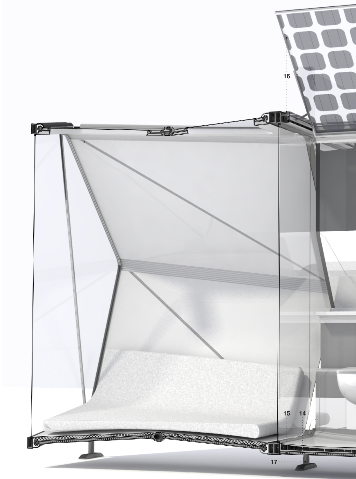
Fig. 5.2.36: a) 3D section - folding units attached to sanitary unit - deployed state
