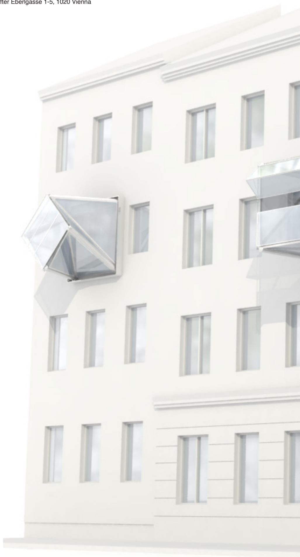
Fig.5.1.02: Facade add-on in different deployment states Facade reconstruction after Eberlgasse 1-5, 1020 Vienna
