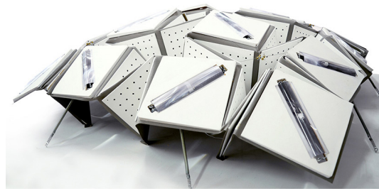
Fig. 4.1.10: Self-adaptive membrane with kinetic nitrinol joints
