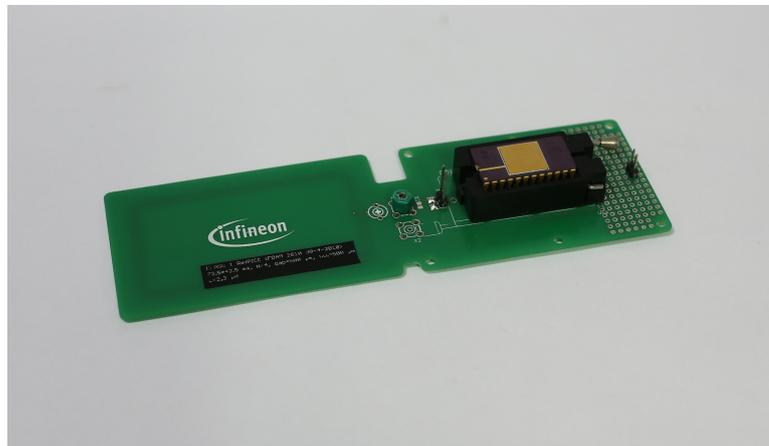
**Figure 8.1:** A reference PICC and a commercial IC, with a variable capacitor added in the middle of the PICC (courtesy of Infineon Technologies Austria AG)
