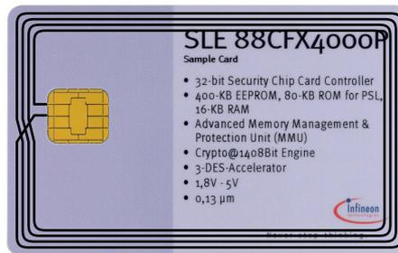
**Figure 2.6:** A contactless chip card (courtesy of Infineon Technologies Austria AG)
