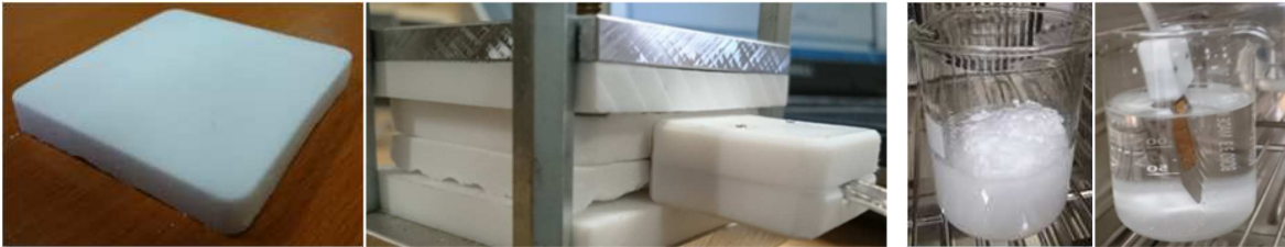
FIGURE 4.11: left: Preparation of two sample blocks and placed foil sensor between the blocks with a defined contact pressure; right: Melting of the PCM in the lab furnace and placed metal frame foil sensor in the PCM liquid
