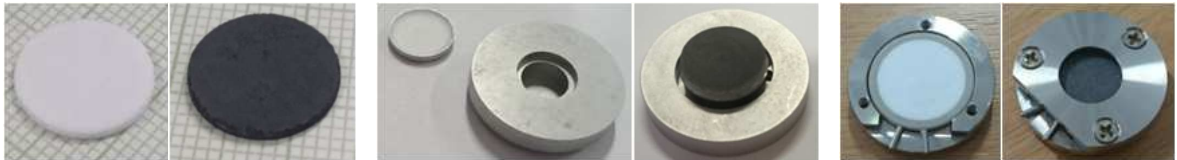
FIGURE 4.9: left: Solid sample in cylindrical shape and graphite coated; middle: Aluminum container for liquids with sample and lid, assembled with graphite coated bottom; right: Polyether Ether Ketone (PEEK) ring with sample inside and steel support outside, assembled with two steel plates on the upper and lower side of the PEEK ring with graphite coating
