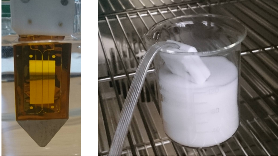
FIGURE 5.18: THB sensor calibration with water and immersed into the powdery sample inside the lab furnace
