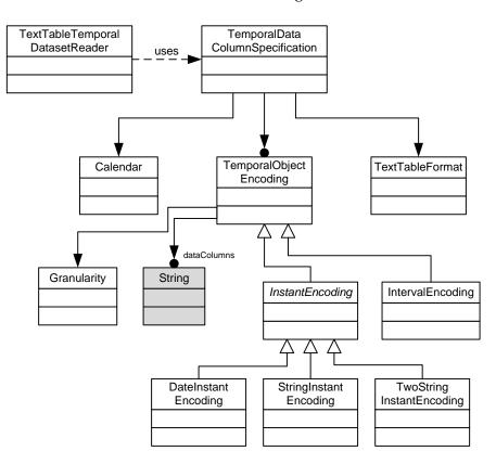
Figure 4.6.: Metadata structure for importing temporal data from CSV text files by the TextTableTemporalDatasetReader: A TemporalObject is created for each line of the input file and each TemporalObjectEncoding with the given data columns. The type of TemporalElement created depends on the subclass of TemporalObjectEncoding. Currently, TimeBench provides three encodings for Instant primitives and one for Interval primitives. All of them allow further configuration.
