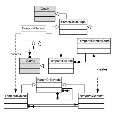
Figure 4.4.: Main data structures in TimeBench: Both TemporalDataset and TemporalElementStore are subclasses of ParentChildGraph, which is a subclass of the prefuse Graph [Heer et al., 2005]. They create TemporalObject and TemporalElement instances respectively. TemporalDataset and TemporalElementStore are linked by an instance of TemporalColumn, which is a subclass of a prefuse Column.
