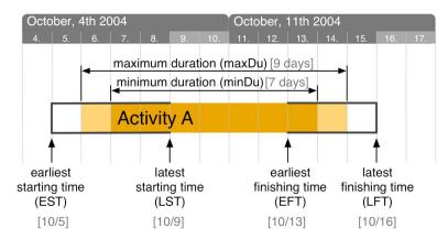
Figure 3.3.: Temporal constraints of the indeterminate interval as represented in the PlanningLines glyph [Aigner et al., 2005] © 2005 IEEE
