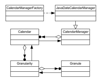
Figure 4.1.: Classes of the calendar package [Rind et al., 2013] © 2013 IEEE The diagram depicts classes and their relations using the extended object-modeling technique [Gamma et al., 1995; Heer and Agrawala, 2006]. The diagram is simplified and does not show all details.
