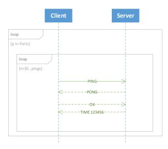
Figure 3.3: TCP4 sequence diagram
