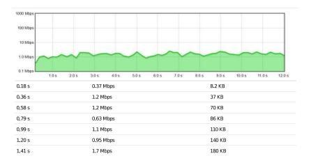
Figure 3.12: Visualization of connection speed during a TCPS4 measurement, generated by netztest.at-code
