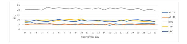
Figure 4.15: Mean TTL values for the traceroutes to *DerStandard.at* during the day (UTC)
