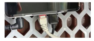
Figure 4.1: Loose contacts of a network cable (white)
