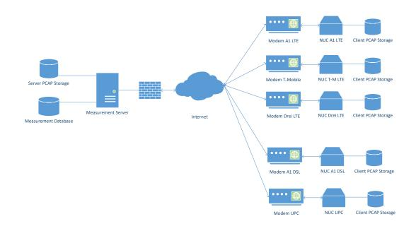
Figure 3.1: Measurement architecture
