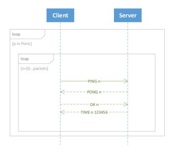
Figure 3.4: UDP4 sequence diagram
