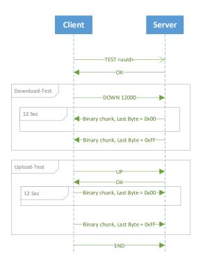
Figure 3.11: TLS4 sequence diagram, following the RMBT specification
