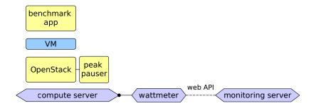
Figure 4.3: Experiment deployment
