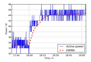
Figure 3.3: An illustration of simple exponential smoothing on a time series of server power consumption samples (obtained from the author's experimental testbed).
