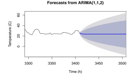
Figure 3.8: Forecasts of air temperature with confidence intervals using AAM.
