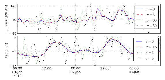
Figure 5.17: Different levels of forecasting errors applied to electricity price and temperature time series (for Mankato, MN).
