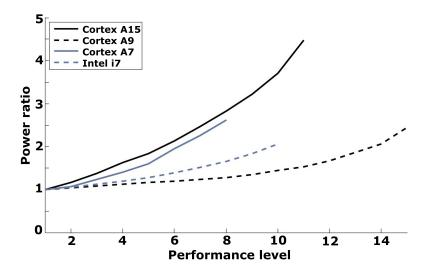
Figure 7.3: Performance to power ratio for different platforms.
