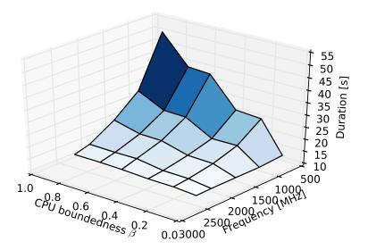
Figure 7.9: Benchmark duration for different workload CPU-boundedness ( $\beta$ ) parameters and server CPU frequencies.
