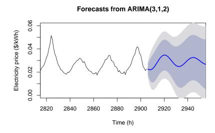
Figure 3.7: Forecasts of electricity prices with confidence intervals using AAM.
