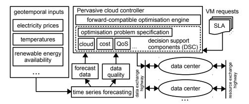
Figure 5.2: Pervasive cloud controller architecture.
