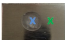
Figure 4.28.: PM-IRRAS measurement positions. Blue cross: on GSH film, green cross: on the Al 2 O 3 surface on the side.
