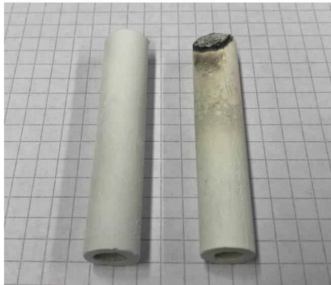
Figure 43: Comparison of a two XP06 samples with 1.0 % SA content and 5 h holding time, left: sintered at 1700 °C, right: sintered at 1750 °C with beginning decomposition
