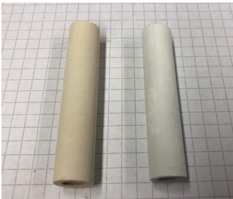
Figure 11: Comparison of the sample before sintering (left) and after sintering at 1700 °C for 5 h (right)
