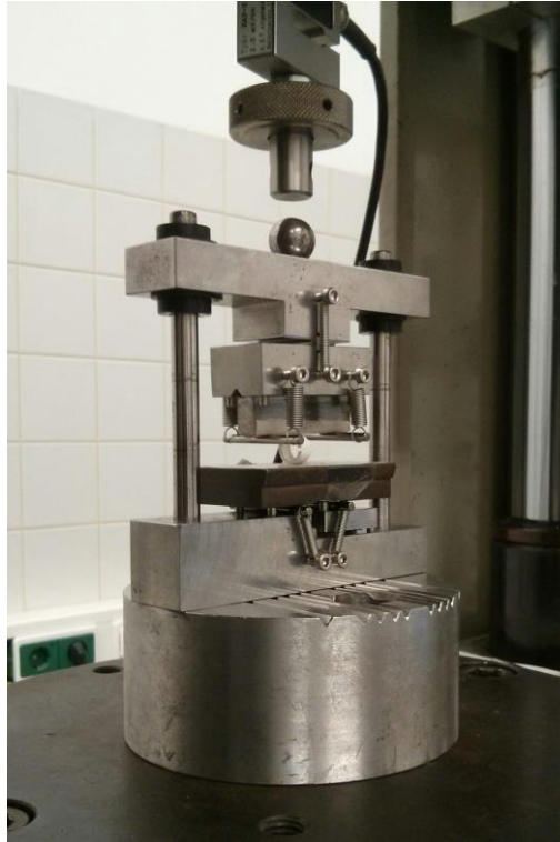
Figure 16: Setup used for compressive strength testing with a built-in C-Ring sample
