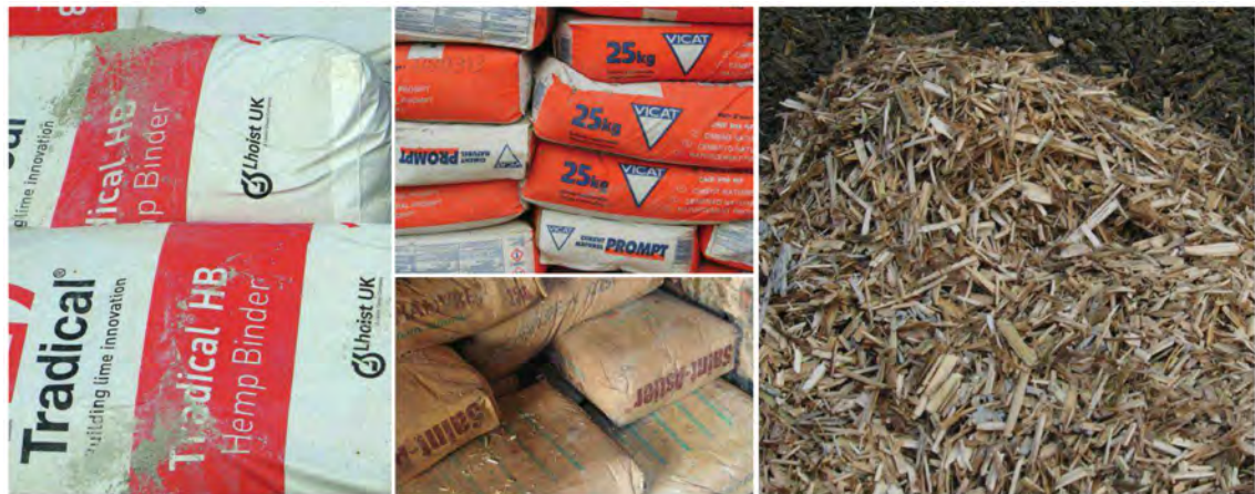
Fig. 29: Most common binders for hempcrete mix, Tradical ® , VICAT and Batichanvre ® (left) and loose hemp shiv (right) (Stanwix and Sparrow, 2014)
