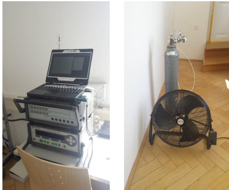
Figure 11 Gas analyzer, SF 6 gas cylinder with pressure reducer and ventilator
