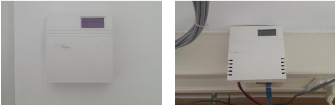
Figure 10 Temperature loggers mounted in the test room
