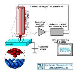
Figure 2.1: Schematical structure of a Scanning Tunneling Microscope (Figure: Michael Schmid, TU Wien)
