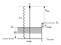
Figure 2.2: Scheme for the determination of the binding energy of a sample (taken from: [10])
