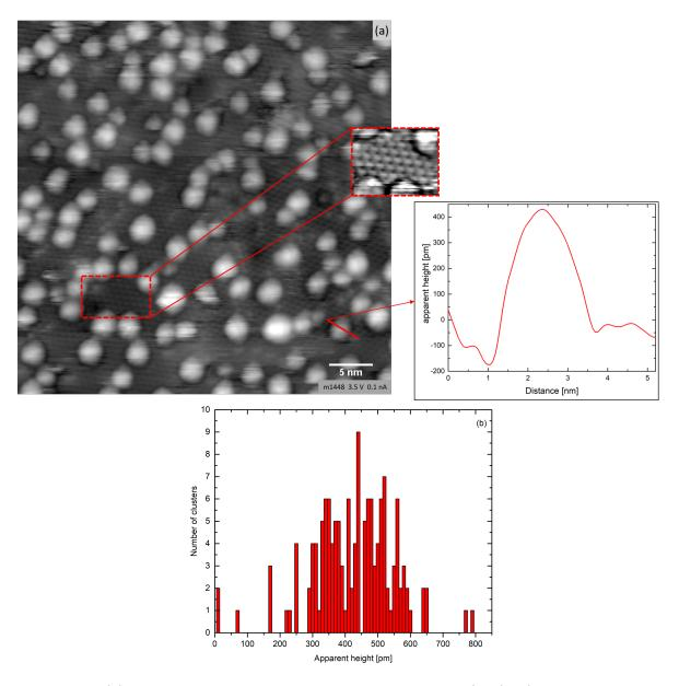
Figure 4.8: (a) STM image of  $0.25 \,\mathrm{ML}$  Fe on monoclinic  $\mathrm{ZrO}_2/\mathrm{Rh}(111)$ . The monoclinic structure is visible (inset). (b) Cluster height distribution.
