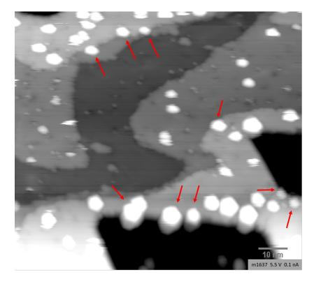
Figure 4.15: STM image of 0.2 ML Ag on monoclinic  $\rm ZrO_2/Rh(111)$ : The clusters tend to grow at step edges (red arrows)
