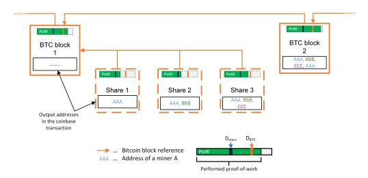
Figure 2.6: Exemplary visualization of the P2Pool sharechain and its connection to Bitcoin. Each sharechain block (denoted as *Share*) references the previous Bitcoin block. With each found share, a new address is added to the outputs of the coinbase transaction of the to-be-found Bitcoin block. Once a full block is found, all miners which have submitted shares receive rewards. In our case miner A will receive half of the generated revenue.
