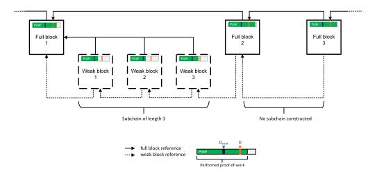
Figure 2.5: Visualization of a subchain between two full blocks. Since each weak block was initially built to become a full block, it has a reference to the previous full block. In addition, all blocks store a reference to the last block of the last subchain. If no subchain is constructed, this reference then too points to the previous full block.
