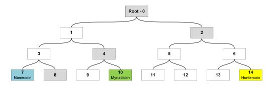
Figure 2.4: Visualization of a Merkle tree used when merge-mining multiple child cryptocurrencies in parallel. For Namecoin to be able to verify that the respective block hash is contained in the Merkle tree at position 7, hashes of the fields 8, 4 and 2 (coloured in grey) must be provided in addition to the root hash (0). Furthermore, the order in which to apply the given hashes (in our case "right", "right", "right") must be included.
