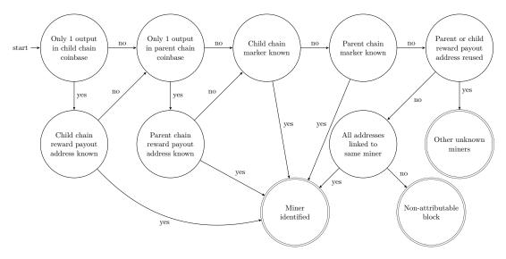
Figure 3.3: Block attribution scheme for merge-mined blockchains utilizing coinbase markers and payout addresses of both parent and child coinbase transactions for identification. Applied to Namecoin, Dogecoin, Huntercoin and Myriadcoin in our study.
