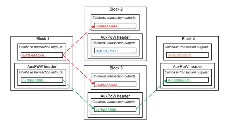
Figure 3.1: Simplified visualization of intersection detection between parent ( $\theta x1BBB$  and  $\theta x1CCC$ ) and child chain ( $\theta xMAAA$  and  $\theta xMDDD$ ) reward payout addresses.  $\theta x1CCC$  and  $\theta xMDDD$  represent newly identified address of the miner/mining pool associated with addresses  $\theta x1BBB$  and  $\theta xMAAA$ .
