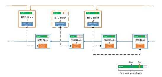
Figure 2.3: Overview of merged mining in Bitcoin with Namecoin. Assuming  $D_{BTC} > D_{NMC}$ , Blocks accepted in Bitcoin will be accepted in Namecoin. However, even blocks missing the difficulty target for Bitcoin, can still meet the requirements for Namecoin, as shown for BTC Block 2'. Furthermore, as depicted for NMC Block 3 and 4, a single BTC block can be referenced my multiple NMC blocks, if numerous solutions meeting  $D_{NMC}$  are found in the process of mining.
