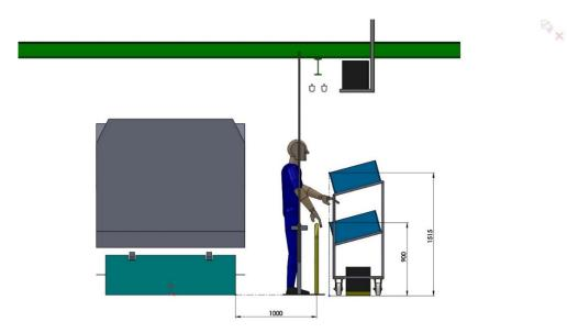
Figure 6.14: Design of overhead conveyor II
