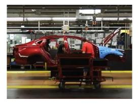
Figure 6.10: Overhead conveyor
