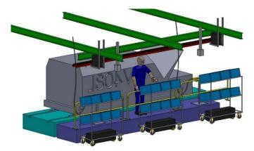
Figure 6.13: Design of overhead conveyor I
