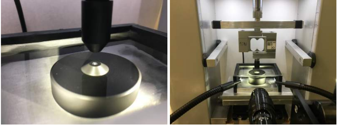
Figure 3.28: The second version of the compression testing set-up
