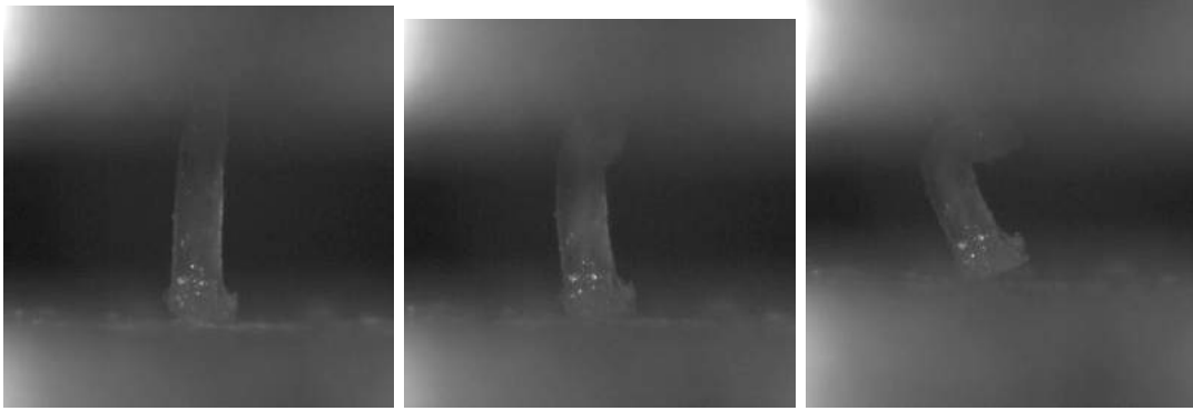
Figure A.2: Images captured during the compression test on osteon # 7 in set-1 with buckling
