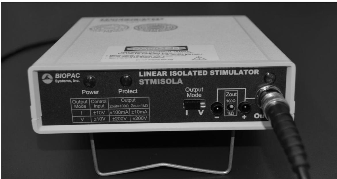
**Figure 4.13: BIOPAC® STMISOLA linear isolated stimulator.** Shown in current mode (I) with high output range of  $\pm 100\ \text{mA}$  ( $Z_{\text{out}} = 100\ \Omega$ ). The cable in the back inputs the control signal, the BNC cable in front is the stimulation output.
