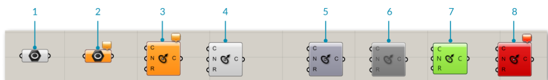
Figure 4-5: Grasshopper colours components based on their functional state.
