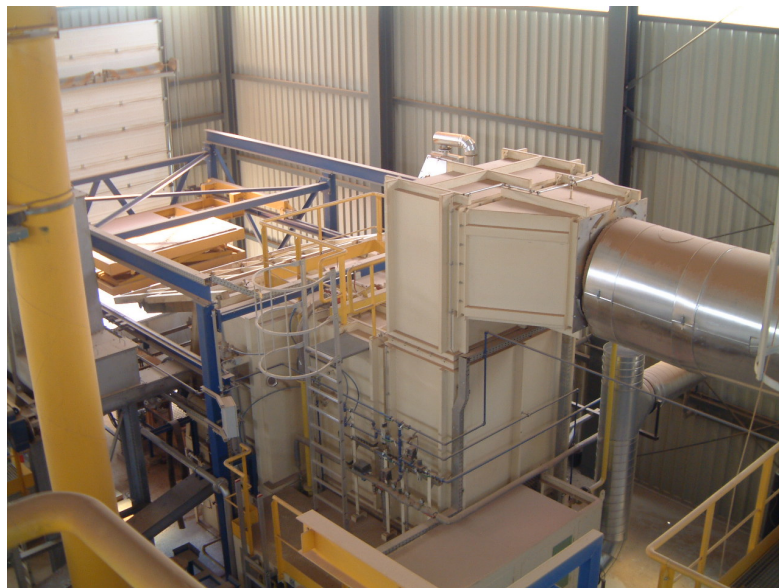
Figure 6.9: The fluidized bed reactor with the attached afterburner chamber
