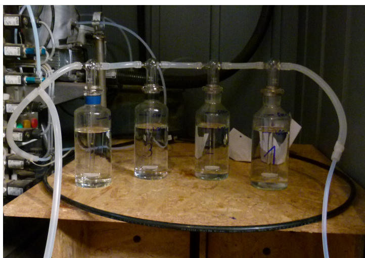
Figure 8.4: Test rig for investigation of the absorption mechanism
