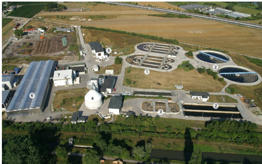
1 main bioreactor, 2 settling tanks, 3 bioreactor for treatment of dairy wastewater, 4 filter press building, 5 digester, 6 greenhouses for sludge drying, 7 sludge incineration plant
