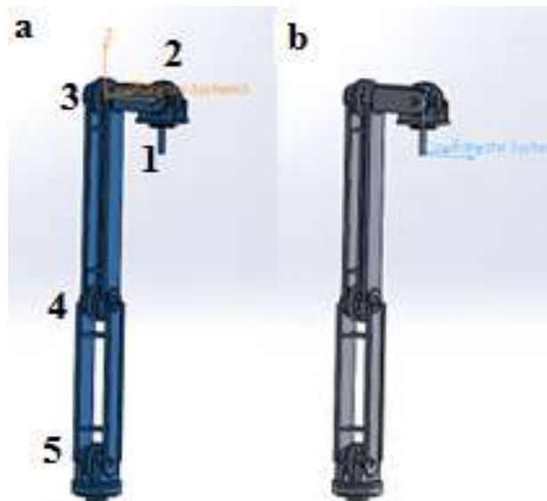
Figure 8-2. Arm with the coordinate systems located on the joint 1 and 3
