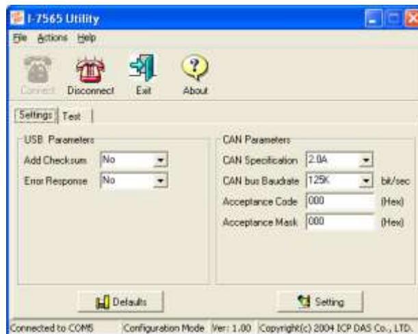
Figure 2-9 Software Utility I-7565 window, (ICP Das (i-7565 Manual), 2007)
