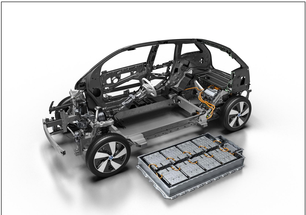
Figure 7: BMW i3 with its main powertrain architecture
