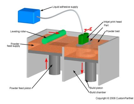
Figure 1.6 – Sketch of the powder-bond binding [6]
