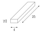
Figure 2.7 – Sample size [mm] for DMA
