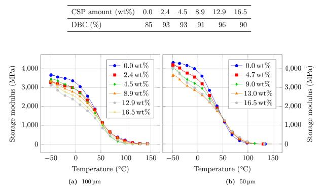
**Figure 3.2** – Evolution of the storage modulus as function of the temperature with different amounts of core-shell particles (commercial resin)
