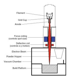
Figure 1.5 – Sketch of the electron beam melting [3]
