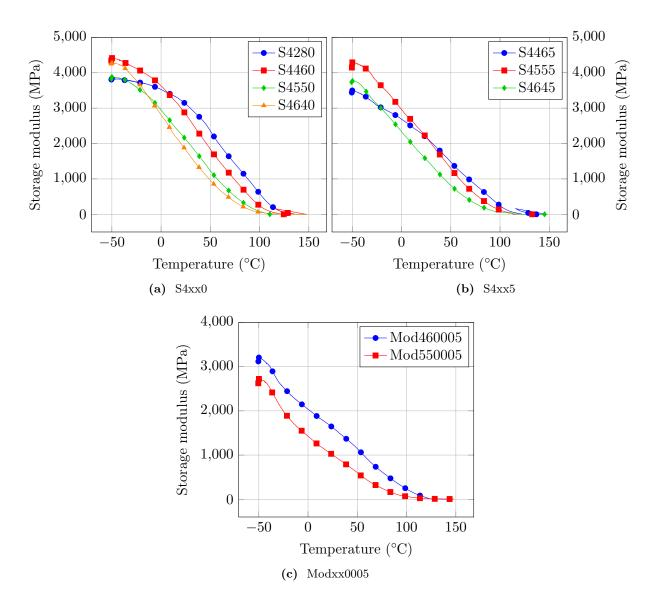
$\label{eq:Figure 3.15} {\bf Figure ~ 3.15-Evolution~of~the~storage~modulus~as~function~of~the~temperature~with~different~amounts~of~cross-linker$
