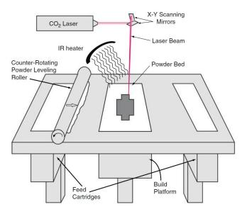
Figure 1.4 – Sketch of the selective laser sintering [3]
