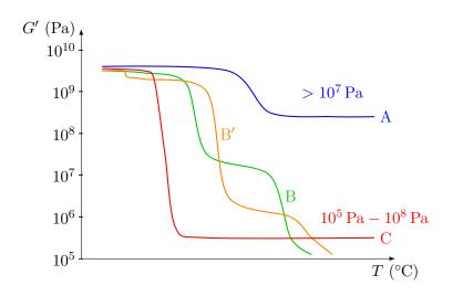
Figure 2.8 – Modulus-Temperature curves for different kinds of polymers [23], [24]
