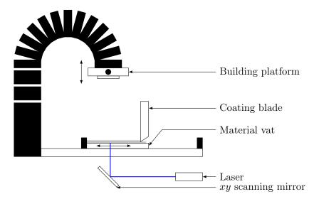
Figure 2.3 – Schematic drawing of the 3D-Printer
