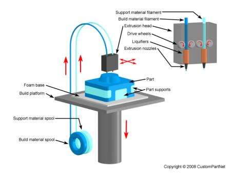
Figure 1.7 – Sketch of the fused deposition modelling [6]
