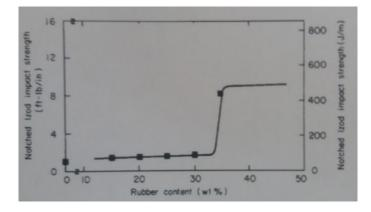
**Figure 1** – Izod impact strength as function of rubber content [1]
