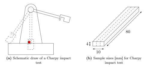
Figure 2.4 – Charpy impact test
