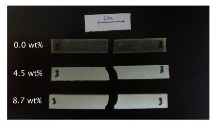
Figure 3.9 – Charpy samples after testing (Mod460000, Mod460005 and Mod460010)
