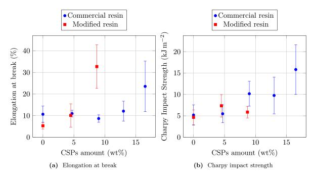
Figure 4.3 – Comparison of the commercial resin and the modified resin (elongation at break and Charpy impact strength)
