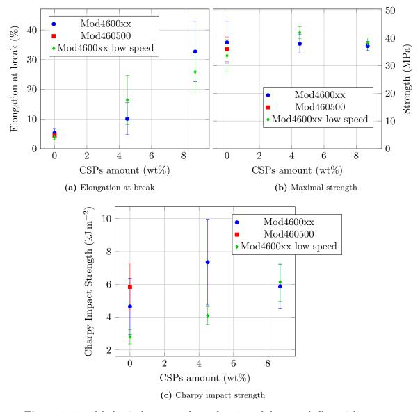
Figure 3.10 – Mechanical tests results as function of the core-shell particles amount (modified resin)
