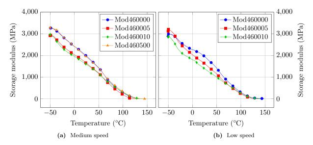
Figure 3.8 – Evolution of the storage modulus as function of the temperature (modified resin)
