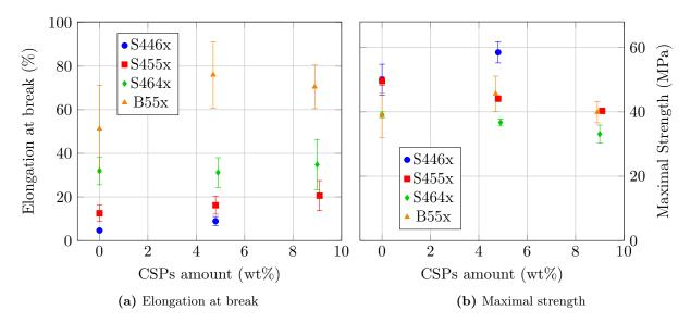
Figure 3.12 – Tensile tests results as function of the core-shell particles amount
