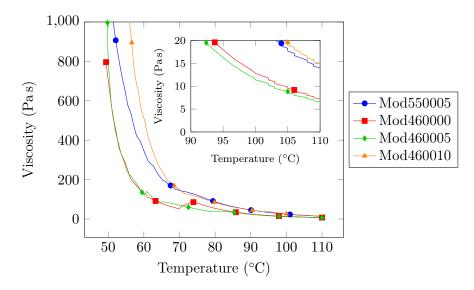
**Figure 3.7** – Evolution of the viscosity as function of the temperature with different amounts of core-shell particles (modified resin)
