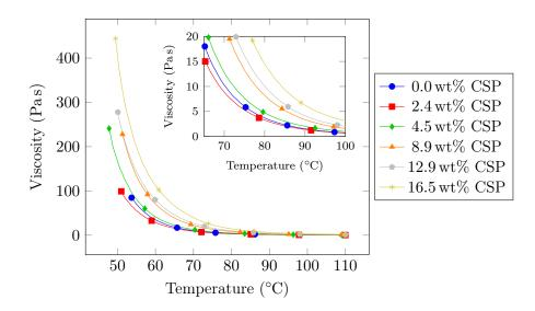
Figure 3.1 – Evolution of the viscosity as function of the temperature with different amounts of core-shell particles (commercial resin)
