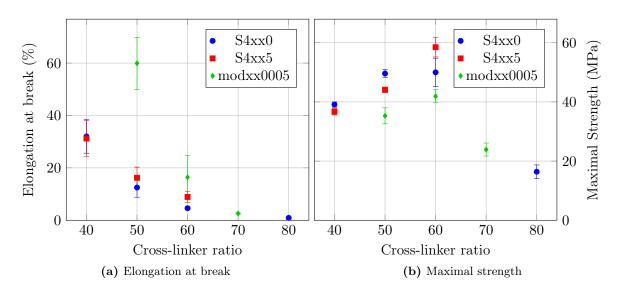
Figure 3.14 – Tensile tests results as function of the ratio between resin and cross-linker
