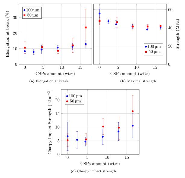
Figure 3.3 – Mechanical tests results as function of the core-shell particles amount (commercial resin)
