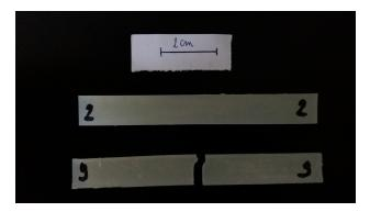
Figure 4.4 – Charpy impact test samples for Mod550005
