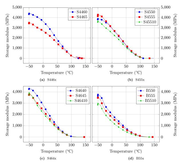
**Figure 3.13** – Evolution of the storage modulus as function of the temperature with different amounts of core-shell particles
