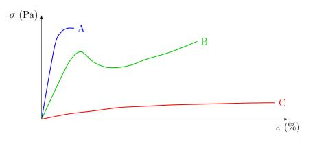
Figure 2.5 – Stress-strain curves for different kinds of polymers [23]
