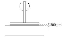
Figure 2.9 – Set-up of the viscosity measurements
