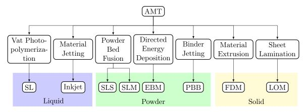
Figure 1.1 – Overview of additive manufacturing technologies [2]
