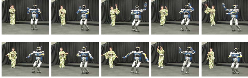
Figure 2.11: HRP-1S performs a Japanese dance which was recorded beforehand with a marker-based motion capturing system [43]
