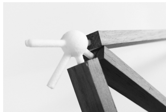
structural model: wooden beams 5/10mm walnut
