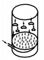
Figure 2.17. perforated plate [51]
