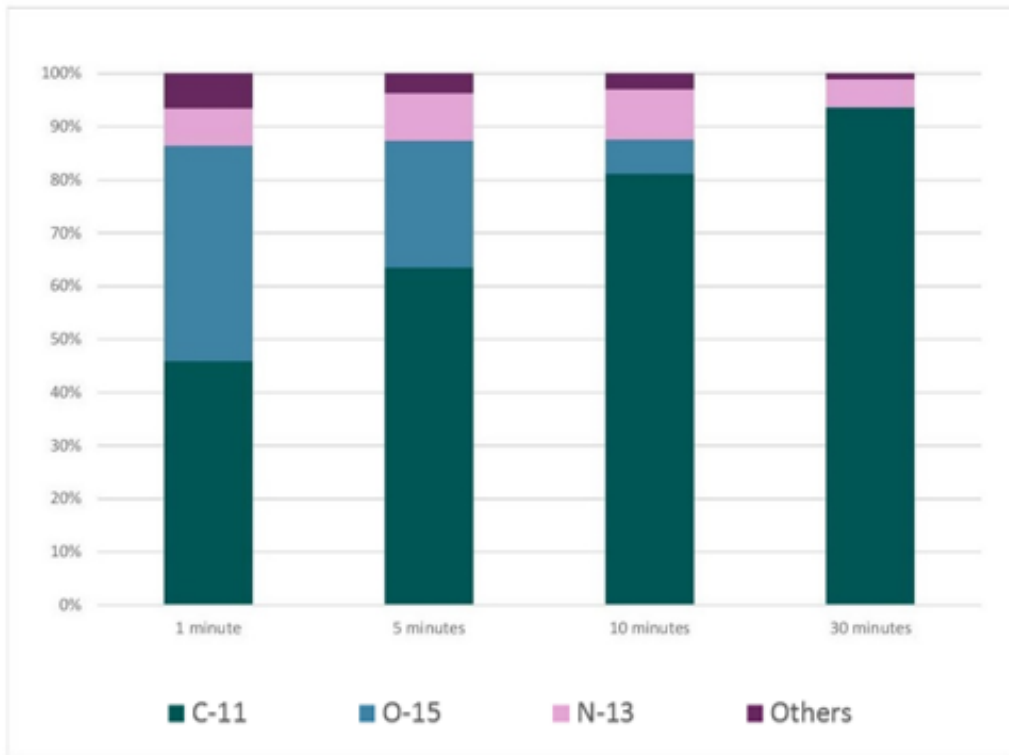
Figure 4.8: Percentage of \beta^+ -emitters over time, 150 MeV, proton beam, 10^7 protons, patient head CT, assuming three minutes irradiation time
