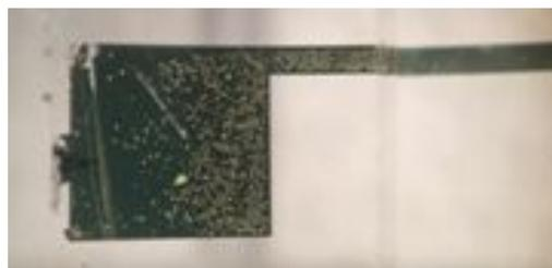
Figure 35.: Not suitable period of time and power of plasma exposure lead to delamination of the electrode.
