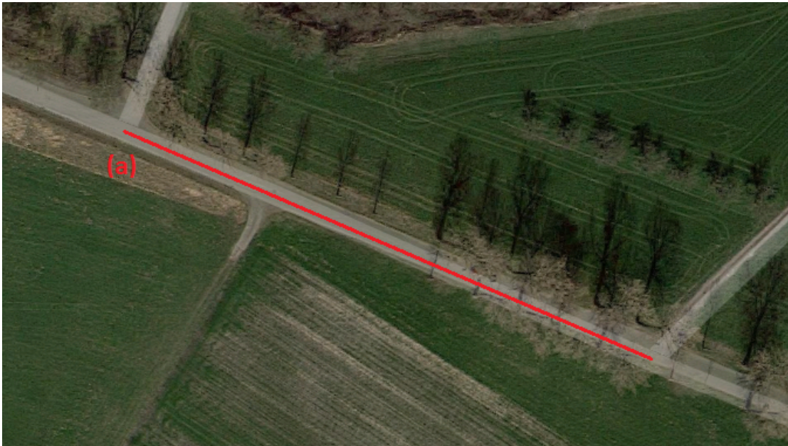
Figure 5.8: Example of an asphalted way which can be clearly distinguished from unpaved surfaces by the image-analysis procedure. The cluster with the brightest RGB values has mean values of 146.8, 149.0 and 131.4, and contains around 40% of the total pixels. The second highest cluster has similar properties and the cluster with the lowest RGB values has mean values of 39.8, 57.6 and 51.4, and a low pixel count. These properties are an indicator for a bright, paved street.
