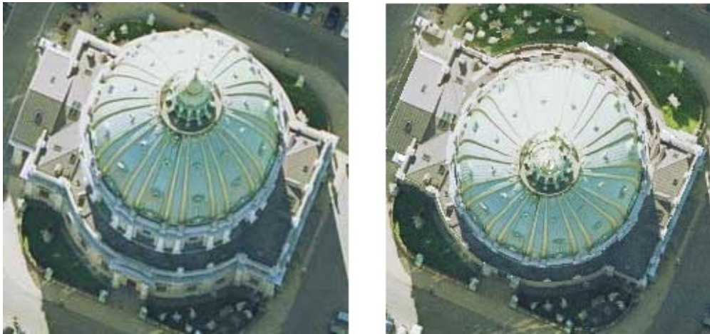
Figure 2.10: Left: Orthofoto before rectification. Right: Orthofoto after rectification. Copyright by Nielsen [dN04].
