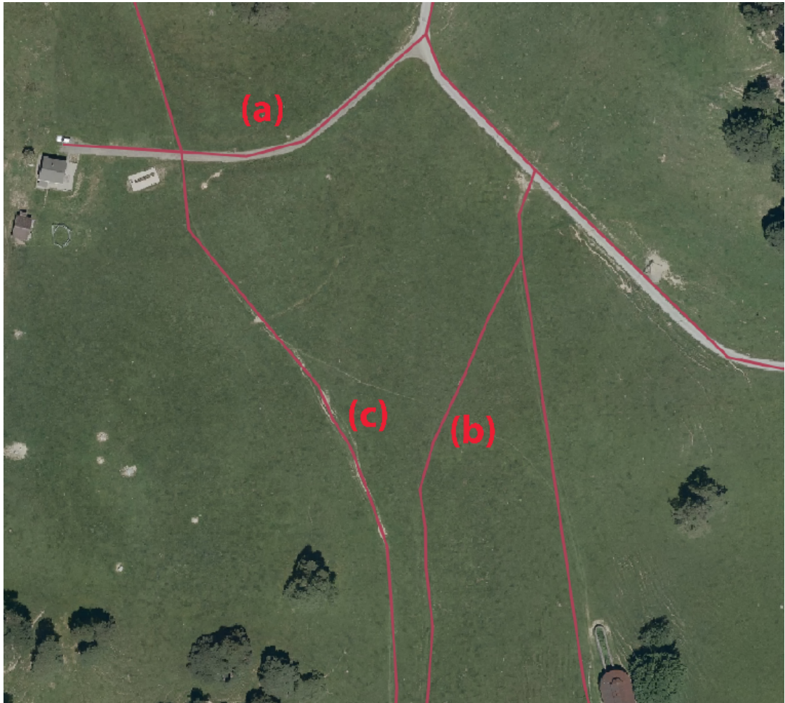
Figure 5.7: Comparison of ways covered with gravel and grass. The way with the gravel surface (a) is visually distinguishable from the ways with the grass surface (b, c), because it consists of much more bright pixels with relatively high RGB values.
