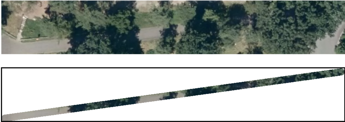
Figure 4.7: An OSM-way occluded by trees before and after extracting it along the “spine” formed by its nodes. Before calculating the spectral signature of the way’s surface, the occluding trees and the actual surface have to be separated, otherwise the result would be biased by the green pixels belonging to the trees. The asphalted areas are not connected because of the trees, which would make floodfill-like algorithms less suited than the k-means algorithm for clustering.
