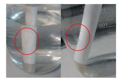
Figure 5 Leakage of the membrane.
