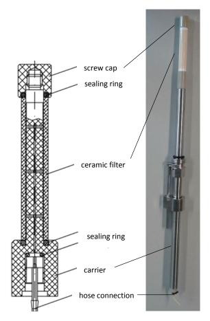
Figure 6 Schematic scheme and picture of a filter membrane.
