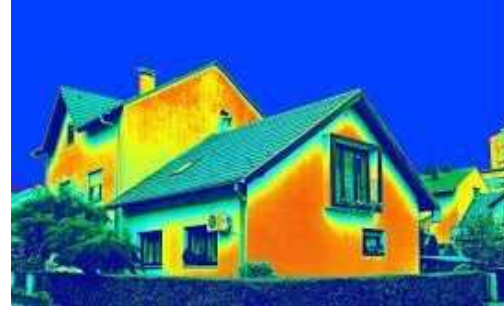
(b) A thermal image of a house with continuous colouring in the rainbow colour-palette. See [54] for more information.
