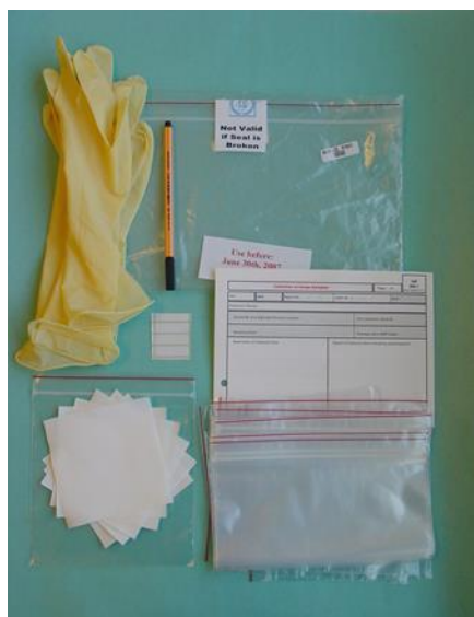
Figure 3: Environmental sampling kit for inspectors
