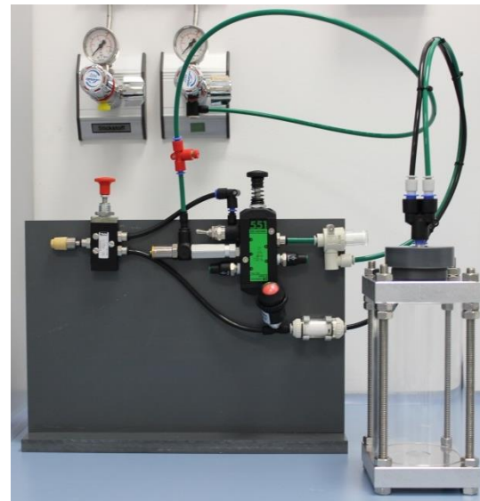
Figure 12: Prototype of explosive-disperser device
