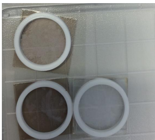
Figure 42: Samples with mica (top and bottom left) detectors and a semadeni plastic.
