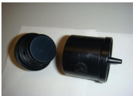
Figure 7: An inertial impactor used at the IAEA Seibersdorf Clean laboratory
