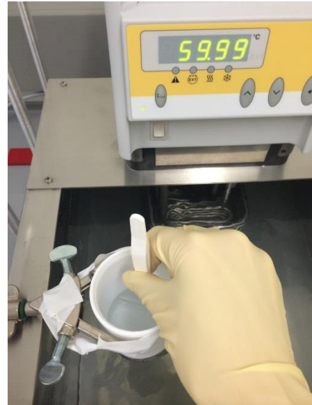
Figure 44: Etching of SSNTD using a forceps. Thermostat bath set to 60°C.
