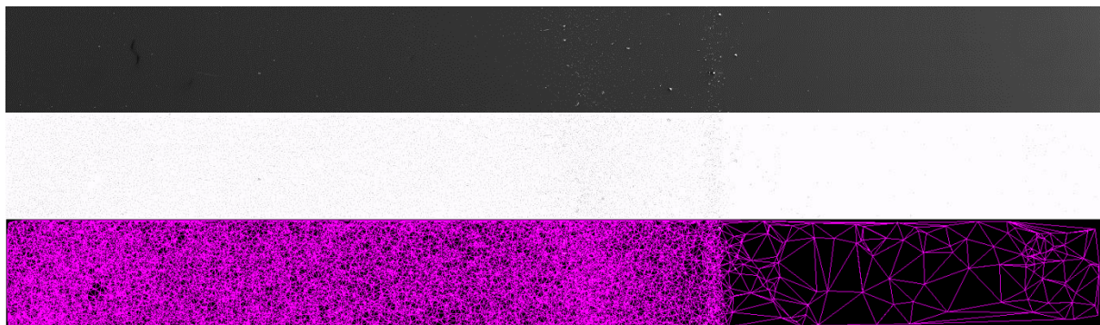
Figure 26: Delaunay Voronoi run on the inertial impactor sample. From top to bottom: segmentation; particle area contouring and triangulation overlay drawing (only centers of mass of particles shown). The mean separation of particles in the outer ring of the inertial impactor sample rises from 40-70 \mu\text{m} to about 570 \mu\text{m} .
