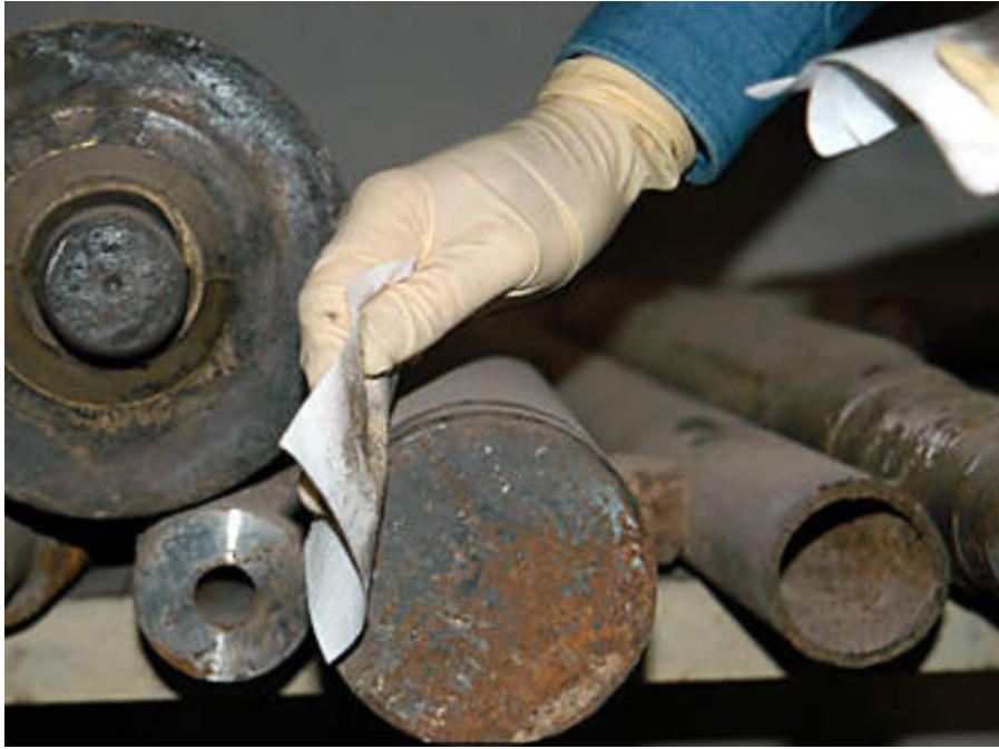
Figure 1: At a machine tool factory, an IAEA inspector takes a swipe sample (as part of the Iraqi nuclear program dismantlement). Photo credits: Pavlicek, IAEA, http://www.iaea.org/newscenter/multimedia/photogallery/photo-gallery-iaea-action-team-inspectors-december-2002
