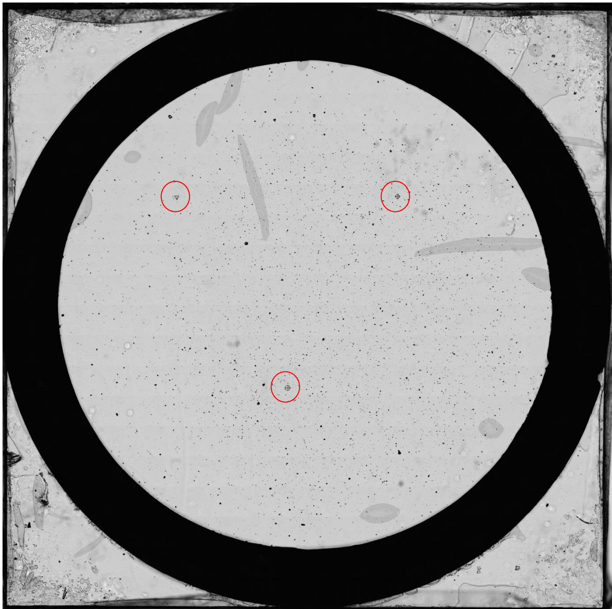
Figure 54: Overview of catcher and detector assembly with three fiducial marks.
