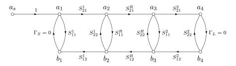
Figure A.4: Signal flow graph of the measurement setup in Fig. A.3.
