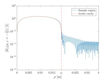
Figure 4.10: M12 model -  $\phi$  component of the normalised magnitude of the electric field for the sample region and for the lower cavity along their interface  $(z = -\frac{d}{2})$ . The radius of the lower cavity  $a_l$  is marked with a dashed vertical line.
