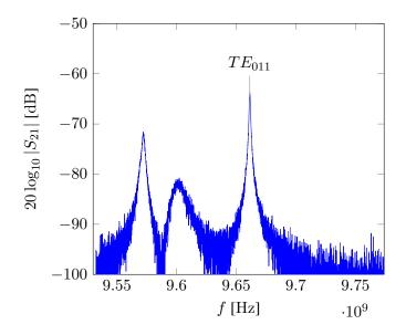
Figure 4.3: Resonance curve of the  $TE_{011}$  mode of our split-cylinder prototype loaded with a 1.509 mm thick PTFE sample. The resonant frequency of the mode was 9.6619 GHz and the quality factor factor was 8754.3, which both were obtained through a circle-fit of the resonance curve.
