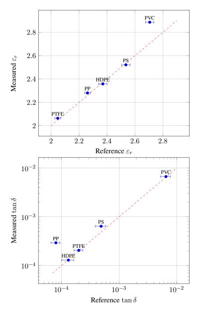
Figure 5.4: Comparison of reference values with complex permittivity measurements for common plastics.
