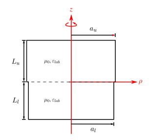
Figure 4.5: Geometry of the asymmetric split-cylinder's calibration model.
