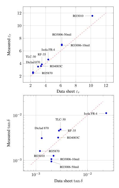
Figure 5.3: Comparison of datasheet values with complex permittivity measurements for microwave substrates.
