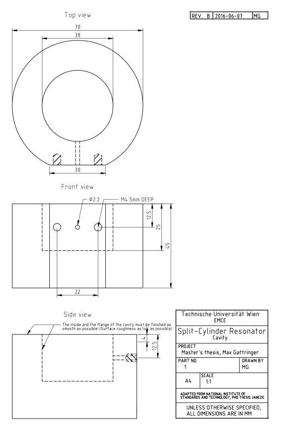
Figure A.5: Drawing of the split-cylinder prototype, adapted from [5].
