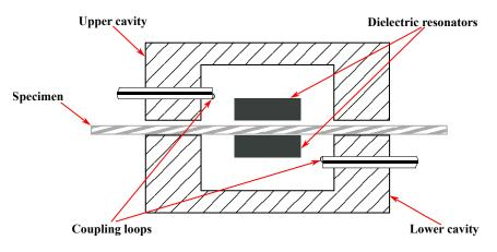
Figure 1.2: Split-post dielectric resonator.
