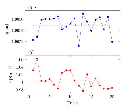
Figure 5.5: Repeatability study of calibration measurements.
