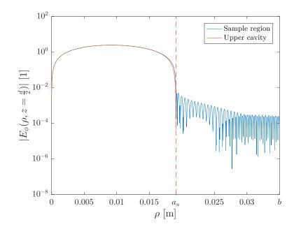
Figure 4.11: M12 model -  $\phi$  component of the normalised magnitude of the electric field for the sample region and for the upper cavity along their interface  $(z = \frac{d}{2})$ . The radius of the lower cavity  $a_u$  is marked with a dashed vertical line.
