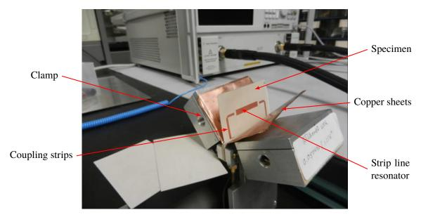
Figure 1.1: Stripline resonator according to IPC TM-650 2.5.5.5c, adapted from [10].
