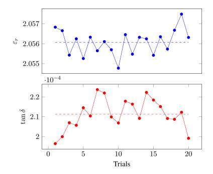
Figure 5.6: Repeatability study of complex permittivity measurements.
