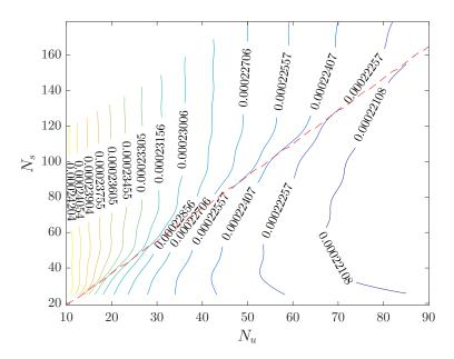
Figure 4.7: Contour plot of the loss tangent of the PTFE sample. The loss tangent is plotted against the number of modes of the sample region  $N_s$  and against that of the upper cavity  $N_u$ . The resonant frequency used for the plot was 9.6619 GHz, the unloaded quality factor  $Q_0$  of the resonance was 8754.3 and the thickness of the sample was 1.509 mm. The dashed line shows the ideal model ratio of  $N_s$  and  $N_u$  according to Il'inksi [48] and Janezic [5].
