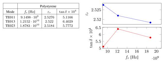
Figure 5.9: Broadband complex permittivity measurement of a polystyrene sample.
