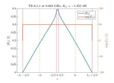
Figure 4.4: The electric field  $E_{\phi}(\rho = \frac{a_l}{2}, z)$  of the TE<sub>011</sub> mode of the sample along the z-axis of the split-cylinder. The sample was a 1.509 mm thick PTFE sample with a dielectric constant  $\varepsilon$  of 2.0563. The plot also indicates the boundaries of the resonator and the location of the coupling loops. As a measure for the coupling of the mode a coupling constant  $K_L$  is shown in the upper right corner of the plot.
