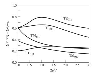
Figure 3.3: Normalized quality factors of cylindrical cavity modes for different cavity geometries, reproduced with permission from [26]. 2a is the diameter of the cavity, and d is the length. The dashed line marks the cavity geometry with the highest normalized quality factor.
