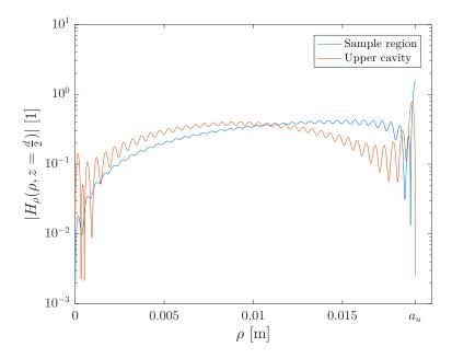
Figure 4.13: M12 model -  $\rho$  component of the normalised magnitude of the magnetic field for the sample region and for the upper cavity along their interface  $(z = \frac{d}{2})$ .
