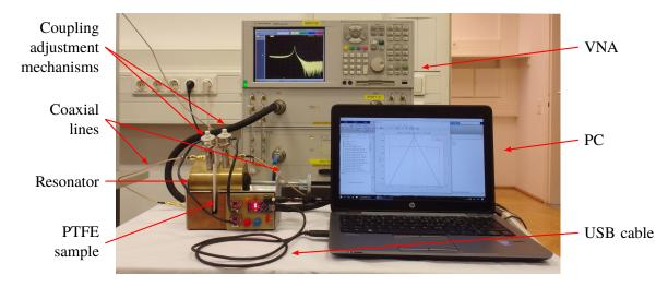
Figure 5.1: Photograph of the measurement set-up.
