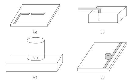
Figure 2.12: Coupling to microwave resonators, reproduced with permission from [26].
