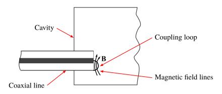
Figure 2.13: Illustration of a coupling loop.
