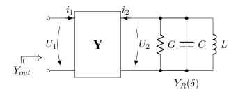
Figure A.2: Input resistance of a two-port coupling network
