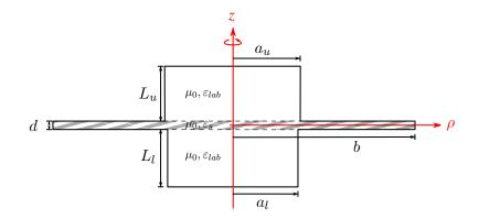
Figure 4.1: Geometry of an asymmetric split-cylinder resonator.
