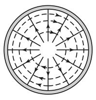
Figure 3.2: Radial magnetic field and azimuthal electric field of the  $TE_{01}$  mode, adapted with permission from [30].
