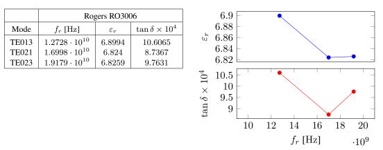
Figure 5.10: Broadband complex permittivity measurement of a Rogers RO3006 sample.
