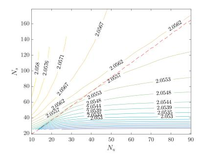
Figure 4.6: Contour plot of the relative permittivity of the PTFE sample. The permittivity is plotted against the number of modes of the sample region  $N_s$  and against that of the upper cavity  $N_u$ . The resonant frequency used for the plot was 9.6619 GHz and the thickness of the sample was 1.509 mm. The dashed line shows the ideal model ratio of  $N_s$  and  $N_u$  according to Il'inksi [48] and Janezic [5].
