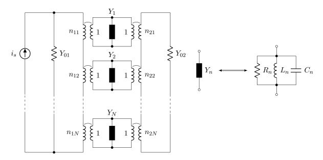
Figure 3.4: Equivalent circuit of the Split-Cylinder resonator.
