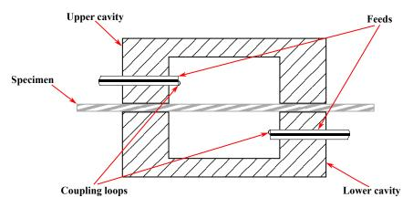
Figure 3.1: Split-cylinder resonator.
