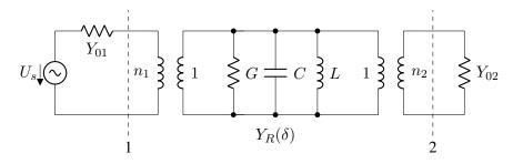
Figure 2.5: Example for a resonator with two coupling networks.
