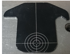
Fig. 5.1: One of the alignment t-shirts. Placed at both ends of the beam expander, those allow for making the beam enter it parallel to the tabletop plane.
