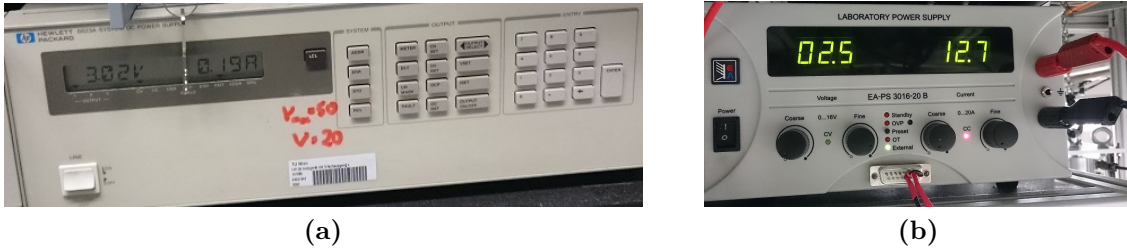
Fig. 4.1: The two current sources controlling the dispensers. Device (a) controls the output voltage of (b) via a Sub-D connector. The dispensers are finally supplied via two banana cables, discernible at the very right.
