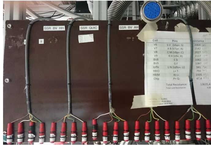
Fig. F.2: Connection board for the superconducting part. By connecting the plug on top to the correct feedthrough, the chip wire and the coils can be manually supplied by an external current source. Primarily, the board is used for monitoring the coil resistances during maintenance work.
