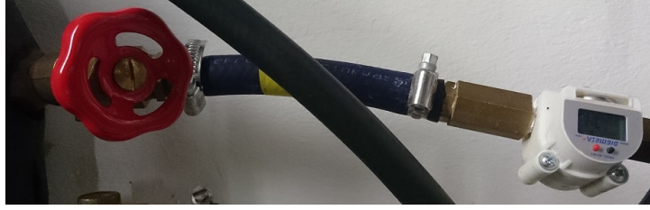
Fig. 4.5: The water cooling valve. This picture is actually flipped by 90^\circ , the valve is located on the left side right after the lab door. It can be distinguished from the other valves by the flow indicator below it. The latter is discernible on the right and should show \sim 8.5\text{-}9.5\text{ l} . In order to prevent leaks due to too strong water flow, the valve should be first opened very carefully and then slowly adjusted to the desired value.
