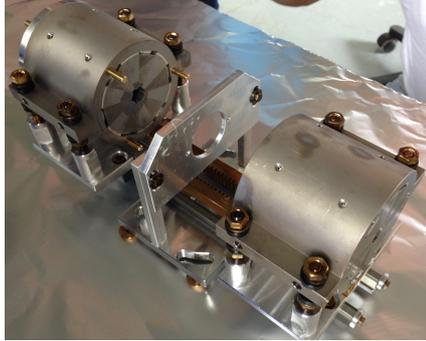
(a) CERN magnets assembly for velocity selection and polarization. The aperture has been removed for this image.
