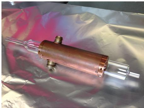
(a) Pyrex tube with radio frequency antenna.
