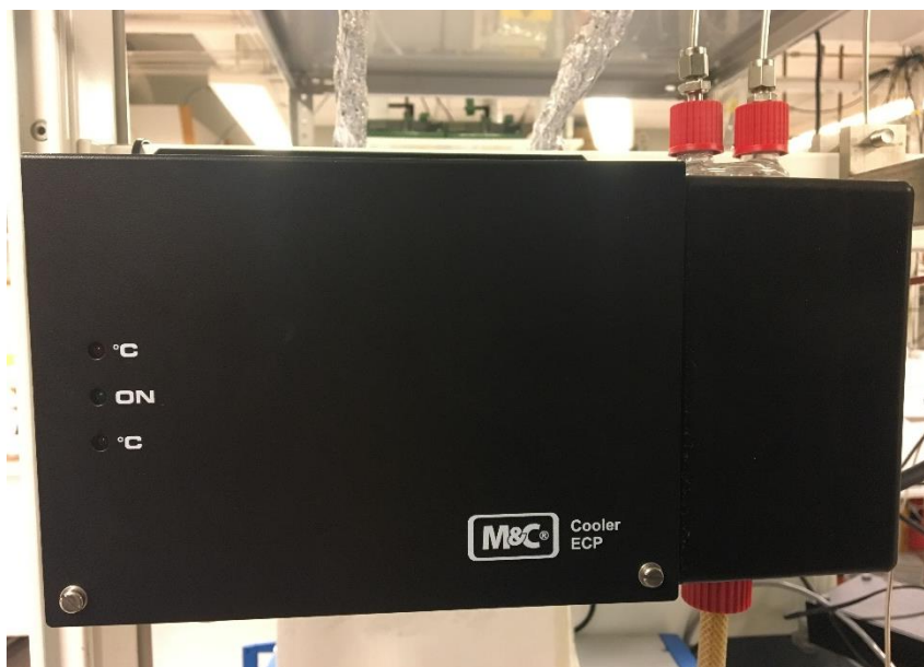
Figure 8: Image of the cooling system used in the experimental setup to cool down the exhaust gas to 5 °C (M&C ECP 3000).
