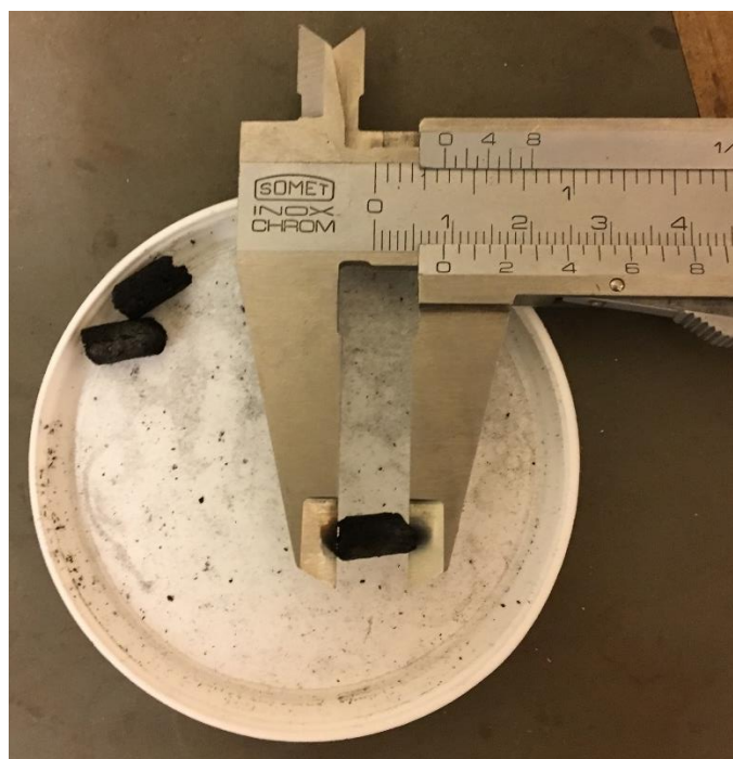
Figure 9: Char pellets used in the experiments with the metal reactor
