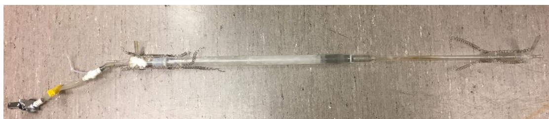
Figure 5: Quartz glass reactor before setting it into the system
