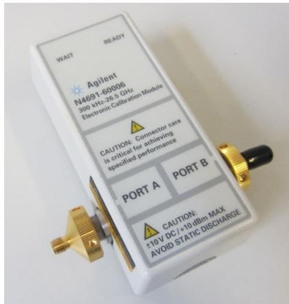
**Figure 1.5: Agilent's electronic calibration module (E-Cal module) allows a mathematical removal of coaxial cables from the setup.**
