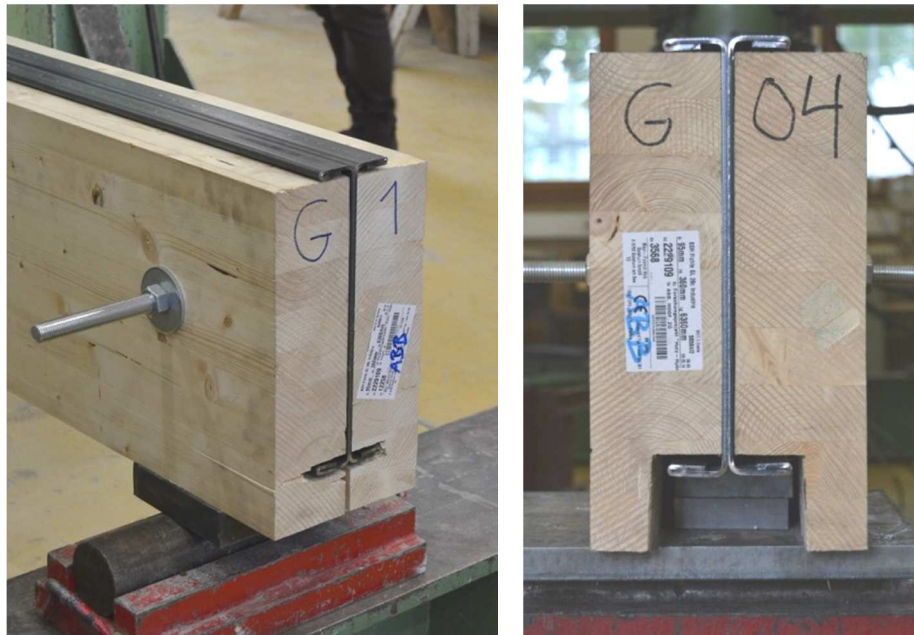
Figure 191: Image of specimens type G from the second testing series, with support conditions “Timber(T)” (left) and “Timber+Steel (T+S)” (right)
