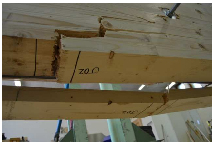
Figure 212: predicted timber ruptures of specimen J02 due to faulty finger-joints
