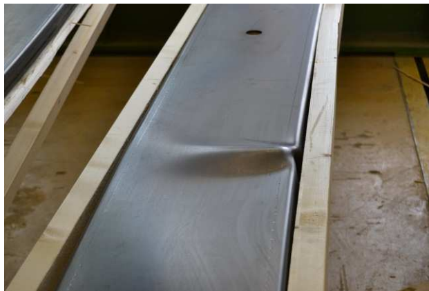
Figure 184: Image of specimen D01 after showing local buckling beginning at the upper steel flange and extending to web
