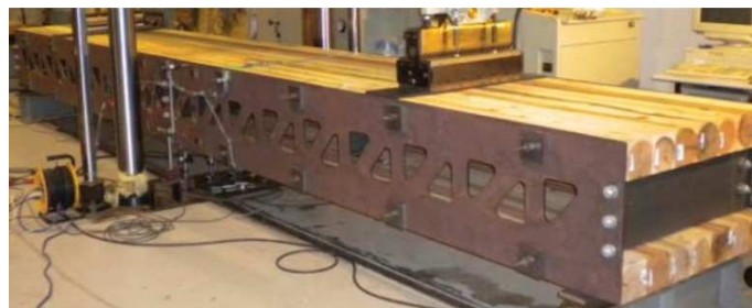
Figure 84: One-box test model with lateral perforated steel plates (122)
