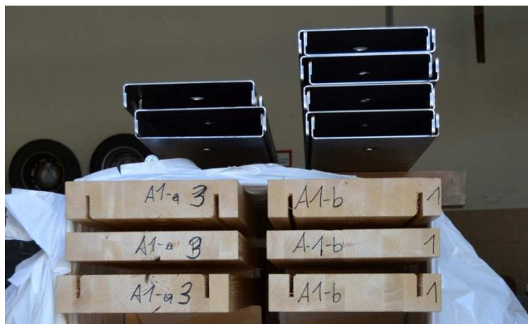
Figure 154: Glulam and steel components for beams before assembling. Beams Type A in the middle of the timber components for the correspondent hybrid beam
