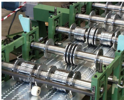
Figure 101: Corrugated sheet steel profile manufactured with roll-forming(216)
