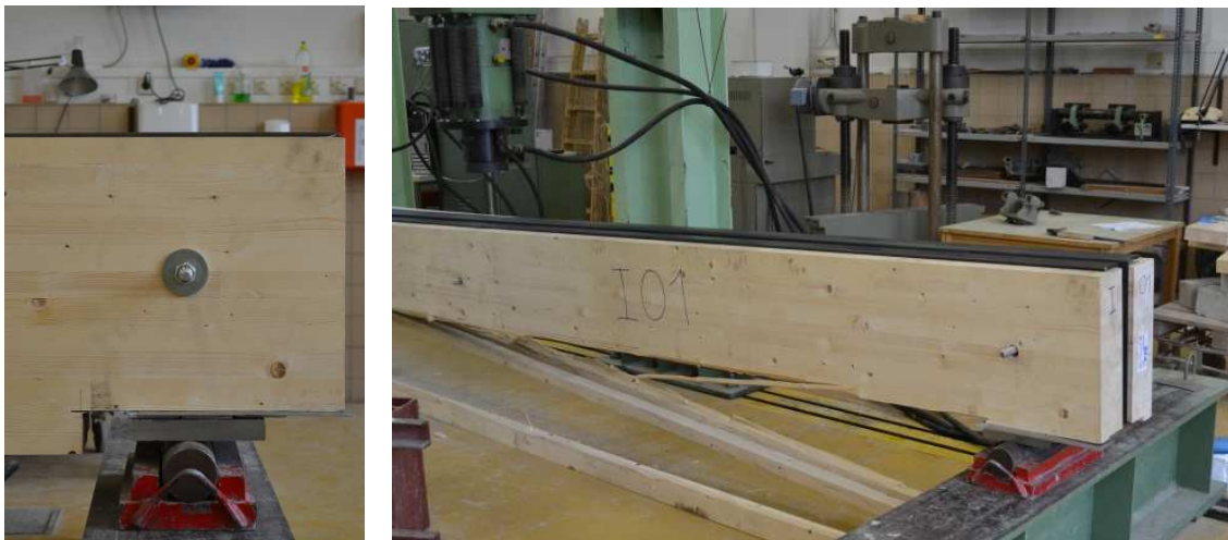
Figure 207: Support of specimen I01 (left) and shear rupture of the same specimen (right)
