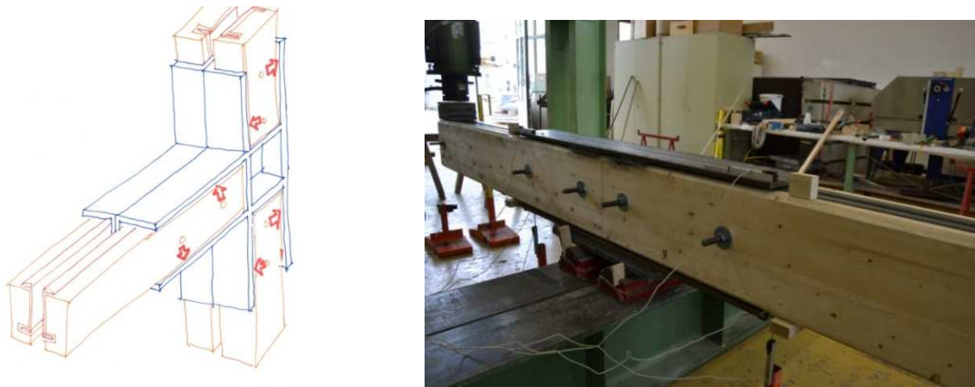
Figure 237: Example of the moment transmission mechanism for knots between timber-steel hybrid beams and supports (left) and testing of a timber-steel hybrid joint (right) (228)
