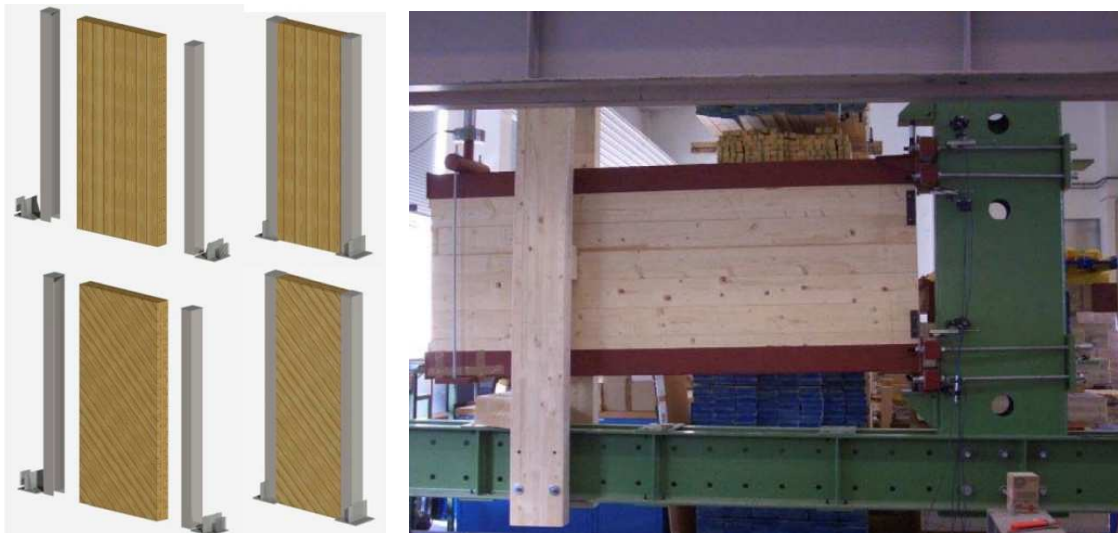
Figure 89: Anchoring system (left) and test set-up for wall and anchoring system (right) (208)
