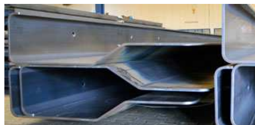
Figure 104: Production (left) of cold-formed steel profiles manufactured with bending presses (right) (217)
