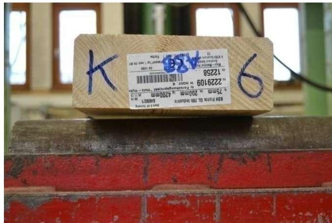
Figure 223: Image where the warping of the specimen K06 can be observed
