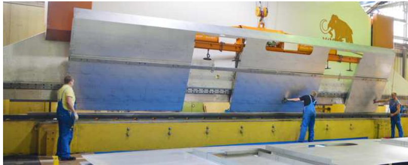
Figure 102: Image of a steel bending press (217)
