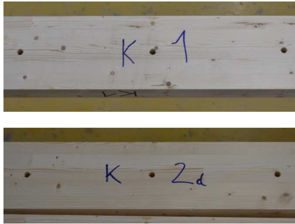
Figure 222: Comparison of the central and bottom face of the beams K01 (rejected due to presence of knots in the middle part and in the proximity to the connecting holes) and K02 (accepted)
