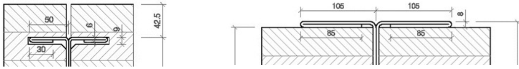
Figure 149: Dimensions of flanges of hybrid beams Type D (left-first testing series) and Type J (right-second testing series)
