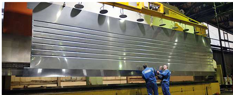
Figure 103: Image of a big-size cold-formed profile (217)
