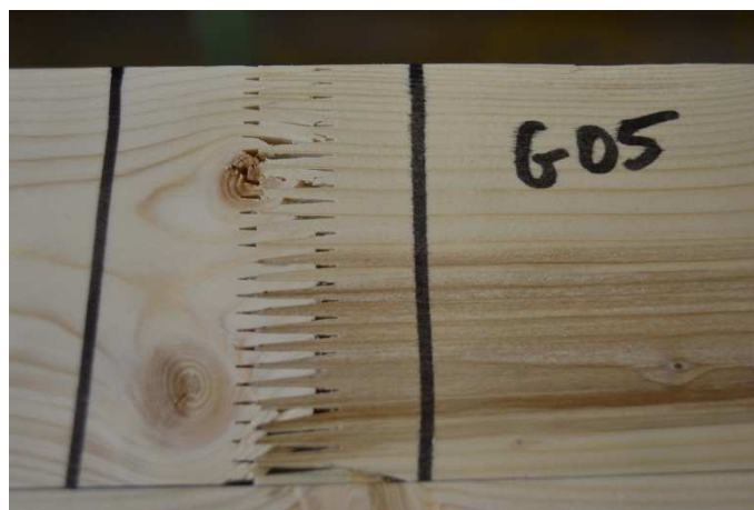
Figure 194: Example of faulty finger-joint in the specimen G05
