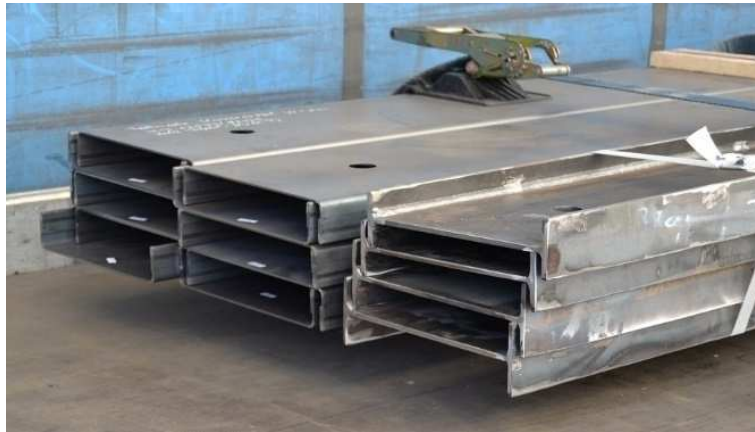
Figure 153: Delivery of steel components, cold formed steel profiles (left) and welded elements (right)
