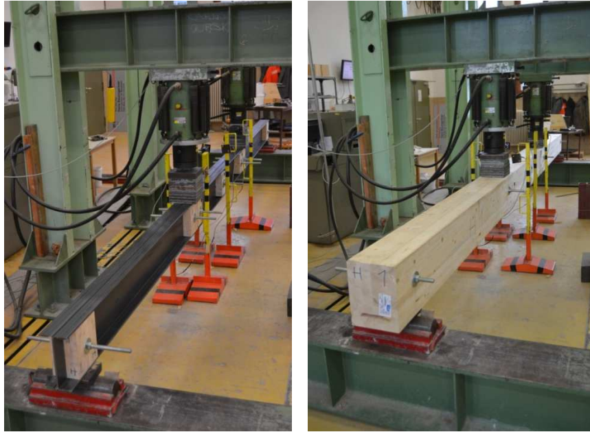
Figure 189: Four point bending test of steel and glulam components of hybrid beam Type H on their own
