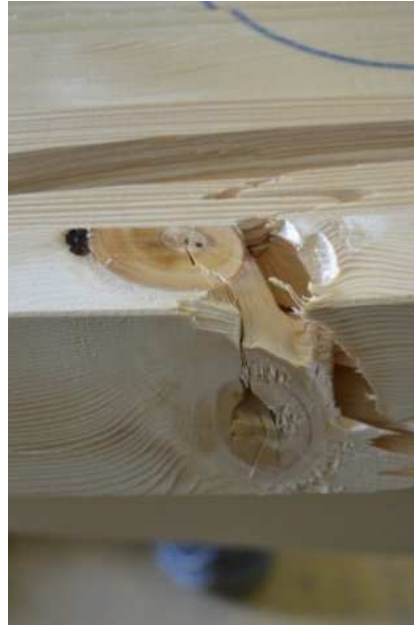
Figure 156: Rupture due to a big knot in the specimen B02
