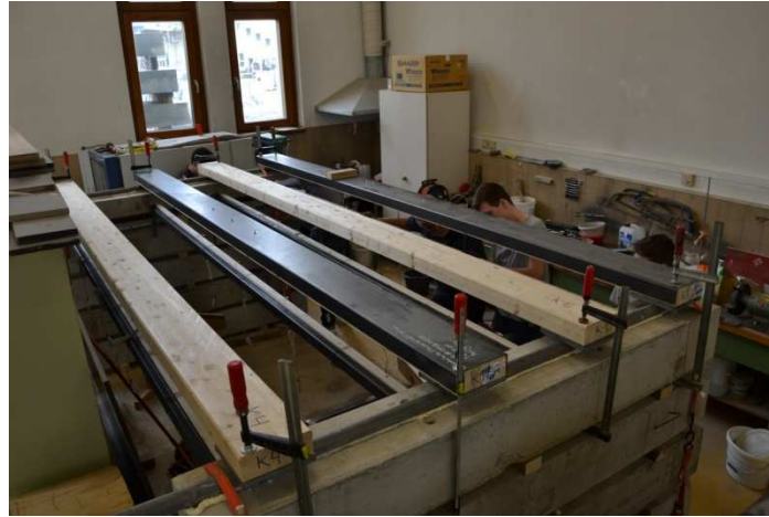
Figure 224: Preparation of the test set-up for the long-term four point bending test
