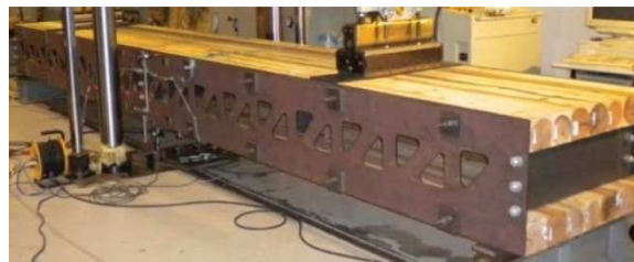
Figure 51: One-box test model (plate) of timber-steel hybrid deck bridge (122)
