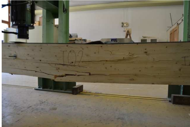
Figure 215: Successive timber ruptures in specimen I02
