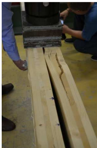
Figure 185: Failure of compression area in specimen Type F
