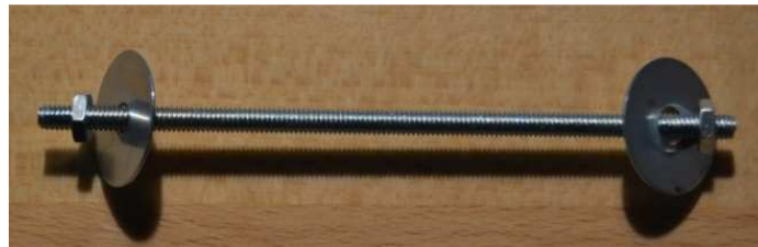
Figure 219: Vertical connector through glulam and steel for the creeping hybrid beams.
