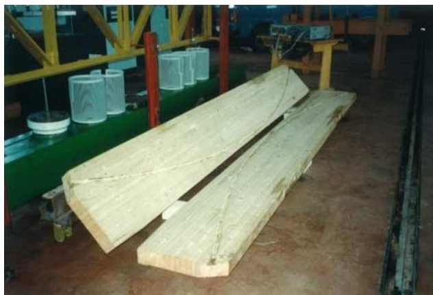
Figure 68: Halves of tested beam with grooves for steel bars (73)
