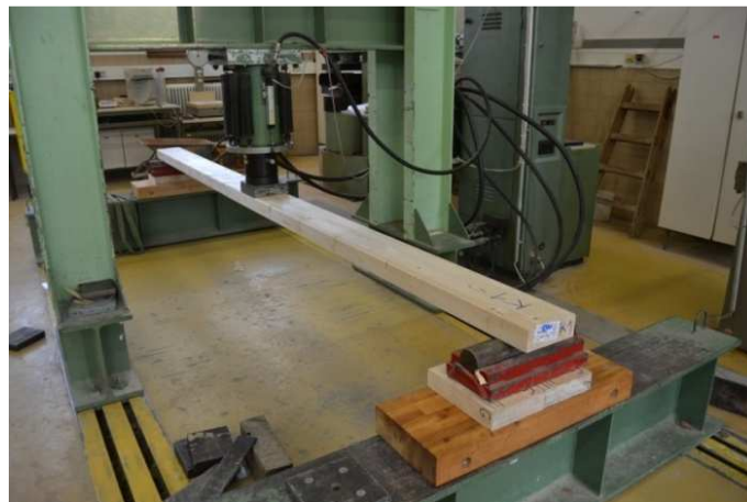
Figure 221: Three point bending tests for selecting the timber specimens regarding their Young Modulus
