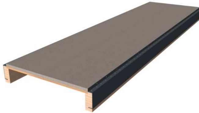
Figure 238: Visualization of a hybrid timber-steel-concrete hybrid ribbed deck prefabricated slab (237)
