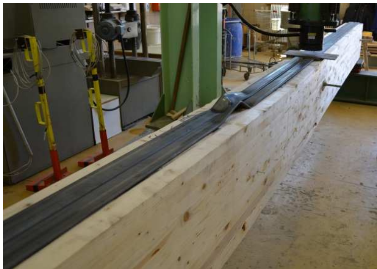
Figure 214: Image of specimen type I showing local buckling of steel flanges after rupture of timber components
