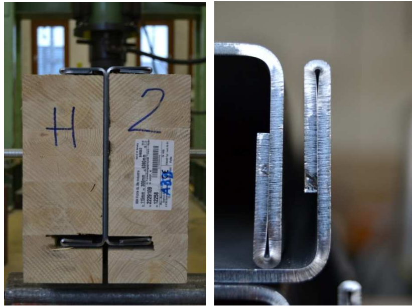
Figure 98: Hybrid beam cross-section and detail of cold-formed steel elements
