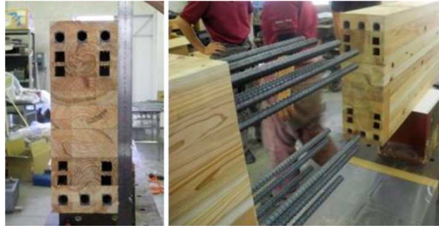
Figure 22: Interface and jointing bars for the moment resisting joints of the RGTSB system (77)
