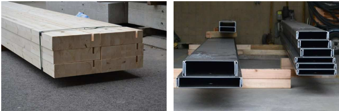
Figure 186: Timber components for beams type G (left) and 8 m and 6 m long steel components (right)
