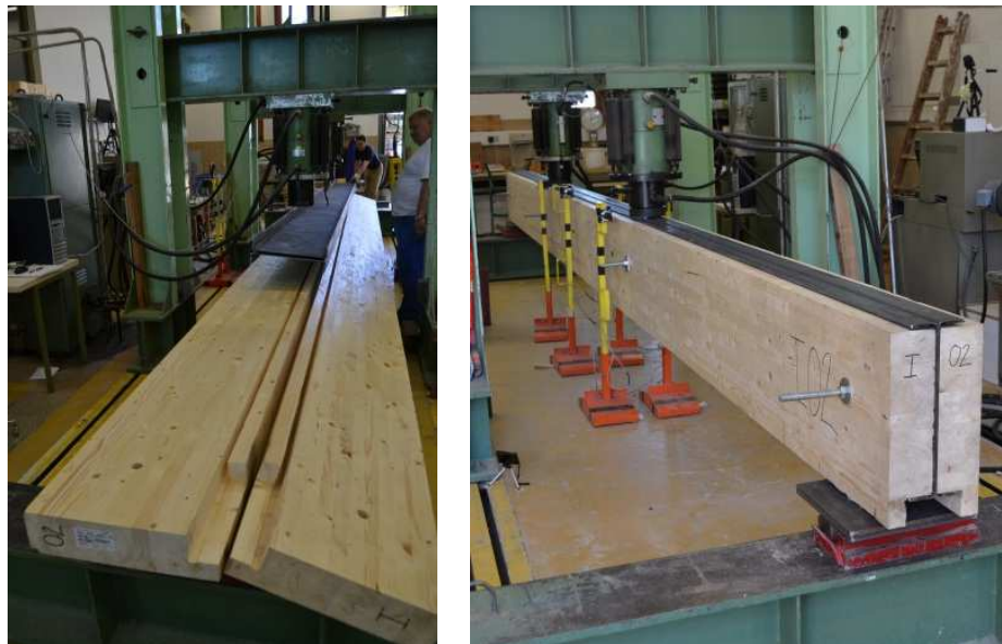
Figure 203: Assembling of 8 metres long specimen I02 (left) and ready for testing (right)
