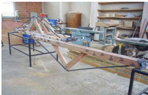
Figure 66: Proposal of pre-stressed beams by Pletz & de Melo Moura (147)
