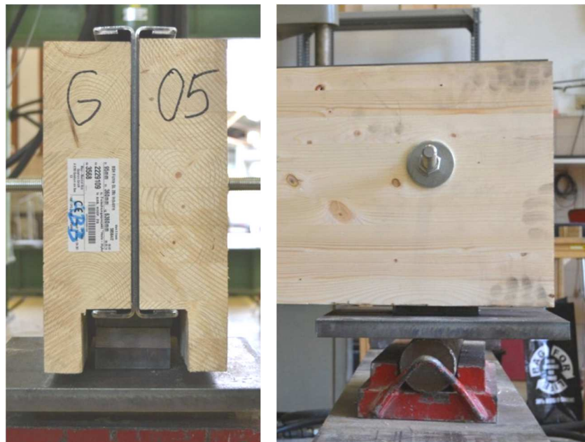
Figure 192: Frontal (left) and lateral (right) images of specimen G05 from the second series, with support conditions “Steel (S)”
