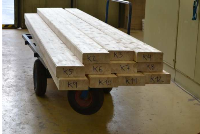
Figure 220: Timber specimens to be tested and classified regarding their Young Modulus values
