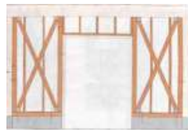
(f) Bracing for bigger openings
