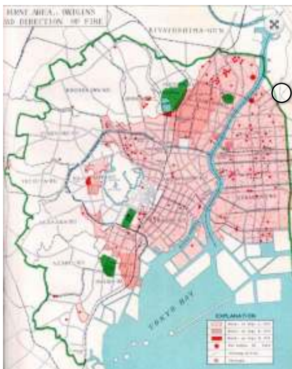
Figure 2.26: Tokyo, Great Kanto earthquake damage, 1923, illustrating origins and extent of fire damage [18]
