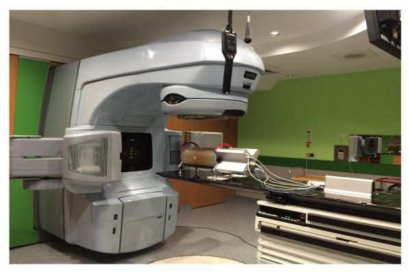
Figure 2.5: Setup for QA plan irradiation at the LKH Wiener Neustadt: the Clinac120 and the Delta<sup>4</sup> phantom.
