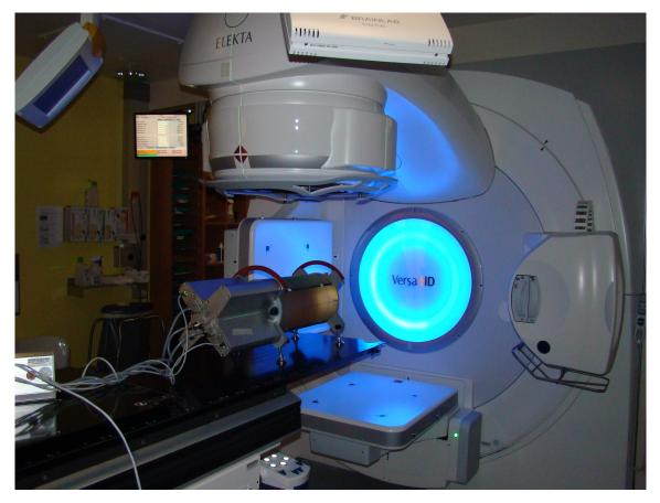
Figure 2.3: Setup for QA plan irradiation at the AKH Vienna: the Versa HD linac and the Delta<sup>4</sup> phantom.
