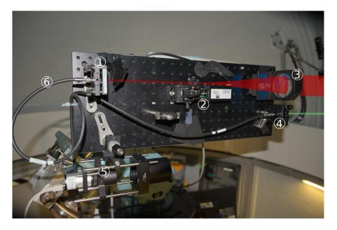
Figure 23: Transmitter telescope. (1) Collimator lens (2) diffuser lens with motorized translation stage (3) Transmitter lens (4) Green collimator lens (5) CCD camera (6) SM fiber
