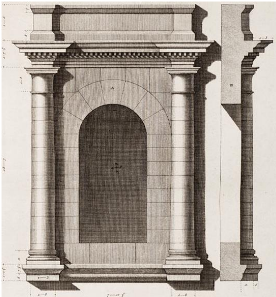
Figure 4.9. Elevation and profile of one arch of the Cryptoporticus, Plate IX, R. Adam
