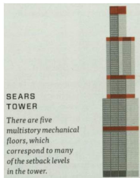
Fig. 86. 5 Mechanical Floors of the Sears Tower
