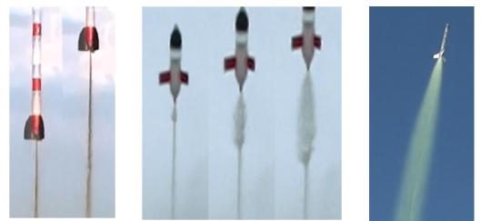
Figure 108: Jet shapes at other rocket models with different nozzle and chamber geometries,  $p_r = 17 \text{ bar}(1)$  Beginning of the flight, using a Laval nozzle (2) The beginning of the air outflow at a simple nozzle (3) Rocket with more smaller chambers and a smaller simple nozzle  $d_2 = 9 \text{ mm}$ .
