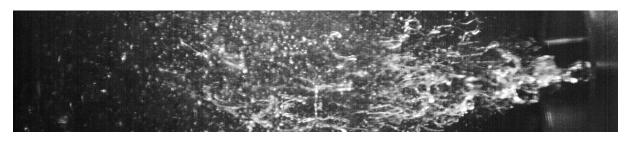
Figure 120: Atomization of paraffin oil at the nozzle
