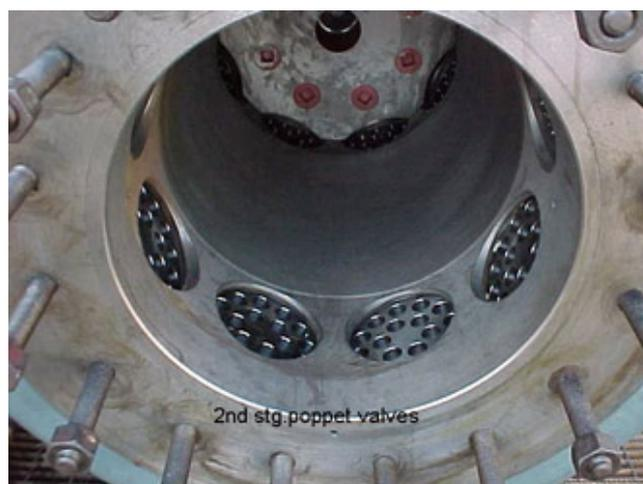
Figure 2.1: Working chamber with removed cylinder head, picture downloaded from the homepage of the John Wood Group PLC [42].
